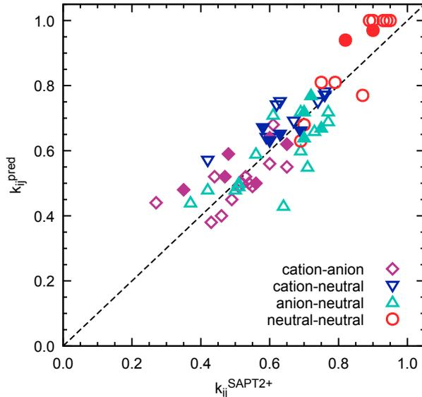
Figure 4: Predicted and SAPT-calculated  $k_{ij}$  scaling factors. Empty points are those used in the original CL&Pol development,<sup>71</sup> whereas filled points are more recent involving new fragments.
