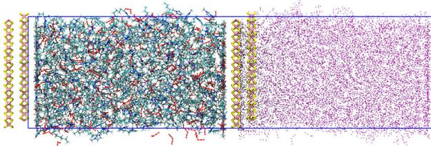
Figure 7: Constant-potential simulation of a substituted imidazolium dicyanamide ionic liquid electrolyte near charged MoS<sub>2</sub> surfaces, with the polarization of the material represented by the image charge method.
