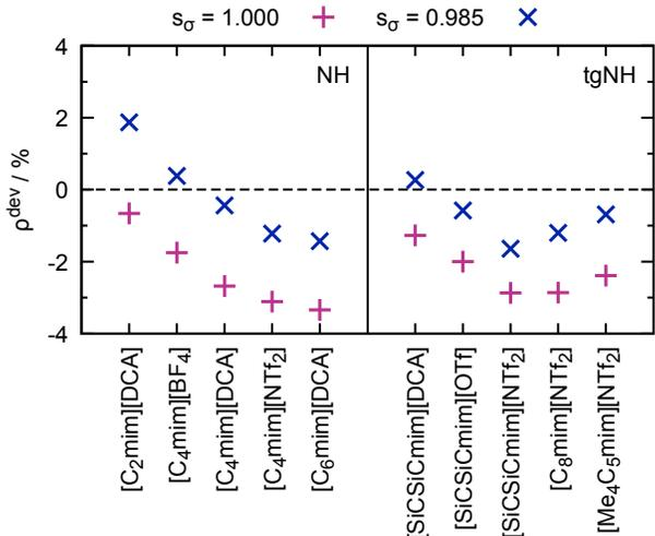
Figure 5: Predicting the density of ILs before and after LJ  $\sigma$  correction by 0.985. NH denotes the dual Nosé-Hoover thermostat, tgNH the temperature-grouped Nosé-Hoover thermostat; SiCSiC corresponds to dimethyl((trimethylsilyl)methyl)silyl)methyl, Me<sub>4</sub>C<sub>5</sub> to 2,2,4,4-tetramethylpentyl side chains in imidazolium cations.
