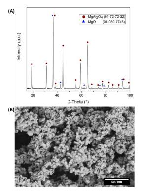
Figure 1: XRD patten (A) and SEM picture (B) of the Reference spinel MgAl<sub>2</sub>O<sub>4</sub> powder.
