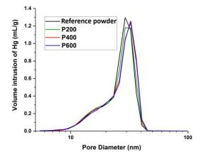
Figure 6 Pore size distributions of green bodies of Reference powder, P200, P400 and P600 green bodies determined by Hg porosimetry intrusion method
