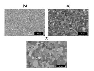
Figure 7: SEM pictures of sintered spinel samples (A) spray dried powder with PEG200 (P200), (B) spray dried powder with PEG400 (P400) and (C) spray dried powder with PEG600 (P600)
