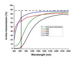
Figure 10: In-line transmission after HIP post-treatment (values normalized to a sample thickness of 2mm)
