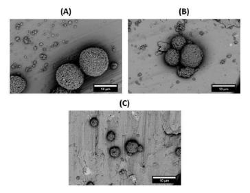
Figure 4: SEM pictures of the spray dried powders P200 (A), P400 (B) and P600 (C)
