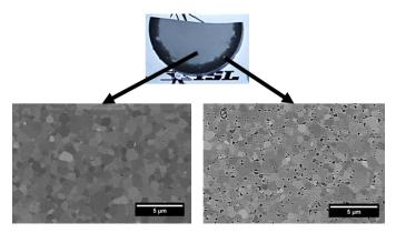
Figure 3 : SEM pictures of the core and rim of the Reference spinel  $MgAl_2O_4$  powder after HIP
