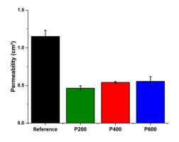
Figure 5 : Permeability at 15kPa of Reference spinel powder, spray dried powder with PEG200 (P200), spray dried powder with PEG400 (P400) and spray dried powder with PEG600 (P600)
