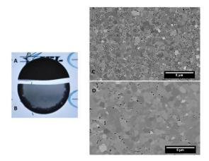
Figure 2: Observations on light table and by SEM of the Reference spinel powder after sintering SRef (A and C) and Reference spinel powder after post-HIP HRef (B and D)
