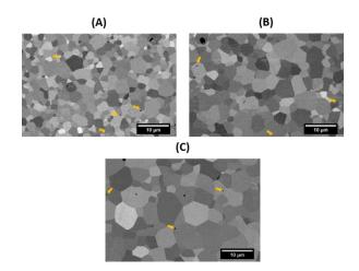
Figure 9 SEM pictures of HIPed spinel samples obtained with (A) spray dried powder prepared with PEG200 (H200), (B) PEG400 (H400) and (C) PEG600 (H600). Pores are indicated by yellow arrows
