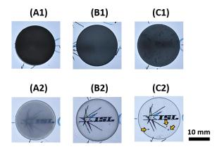
Figure 8: Pictures on light table of (top) sintered ceramics obtained with spray dried powders prepared with PEG200 (Sp200, A1), PEG400 (Sp400, B1) and PEG600 (Sp600, C1) and (bottom) HIPed ceramics obtained with spray dried powders prepared with PEG200 (H200, A2), PEG400 (H400, B2) and PEG600 (H600, C2). Defects are indicated by yellow arrows
