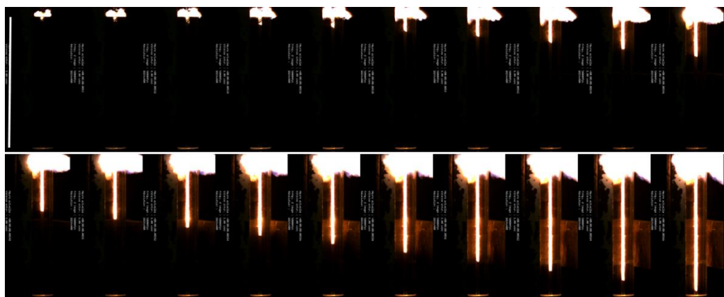
Figure 4. Images captured from the combustion of the Al/In 2 O 3 _nm energetic composite material. The equivalence ratio ( \phi ) was fixed at 1. The elapsed time between images was 40 \mu\text{s} . The white scale bar (at left on first image) represents the tube length (150 mm).
