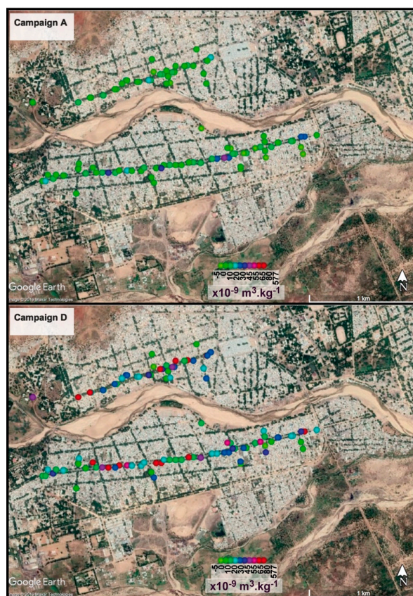
Figure 2. Mass magnetic susceptibility obtained on leaves during campaigns A (mid-August) and D (end-December).
