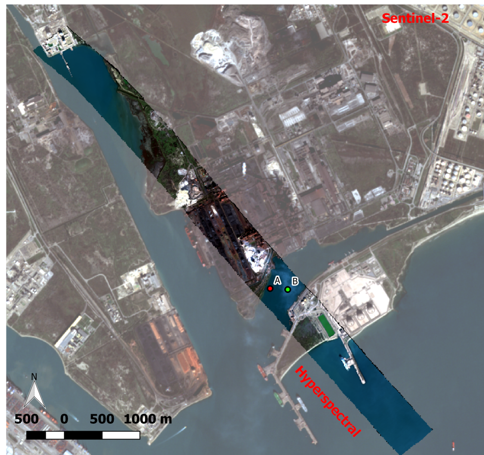
Figure 3. HYSPEX hyperspectral image (opaque) superposed on the Sentinel-2 image (transparent). Points A and B, respectively, represent areas of interest for the spectra used in Figure 7.
