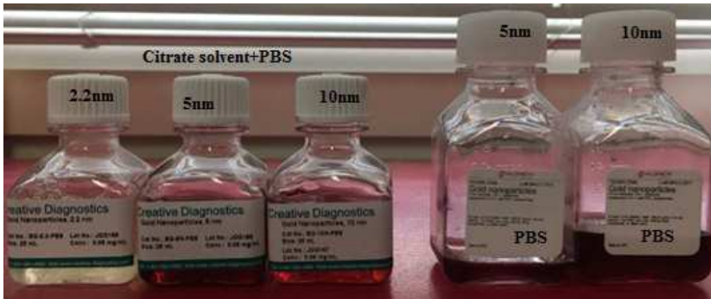
Figure 1. Gold nanofluids of different particle sizes and surfactants coating (PBS and PBS-citrate)
