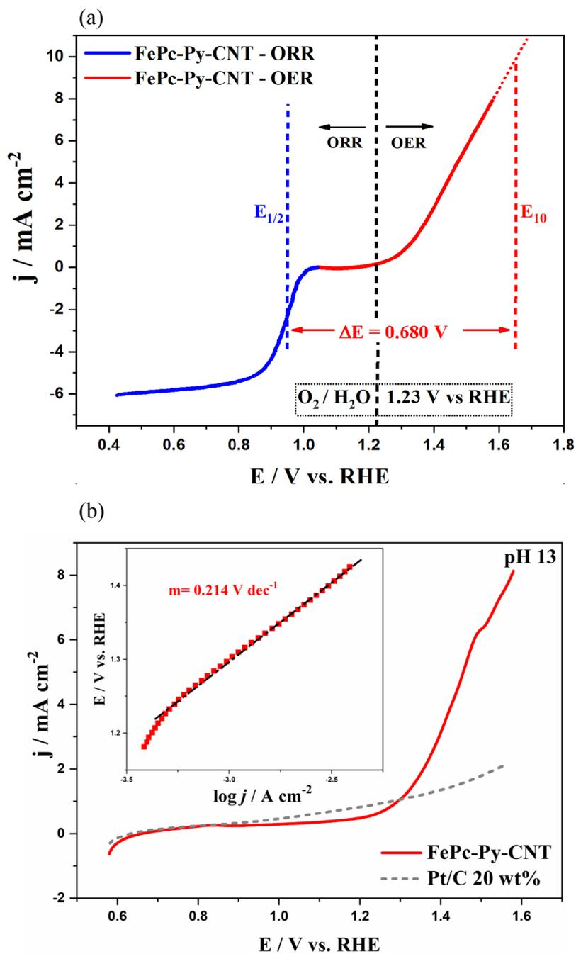
**Figure 4.** (a) Polarisation curves at 5  $\text{mV s}^{-1}$  for ORR and OER in 0.1M KOH with FePc-Py-CNT catalyst. (b) polarisation curve at 5  $\text{mV s}^{-1}$  in deaerated 0.1M KOH solution and inset with Tafel plot for OER.
