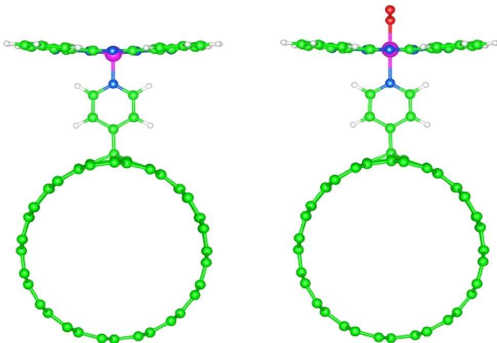
**Figure 7:** Computed structure of FePc bound to carbon nanotubes through amino pyridine linkages, with and without the presence of molecular oxygen, and using blue, purple, red, and green colour for nitrogen, iron, oxygen, and carbon atoms respectively.
