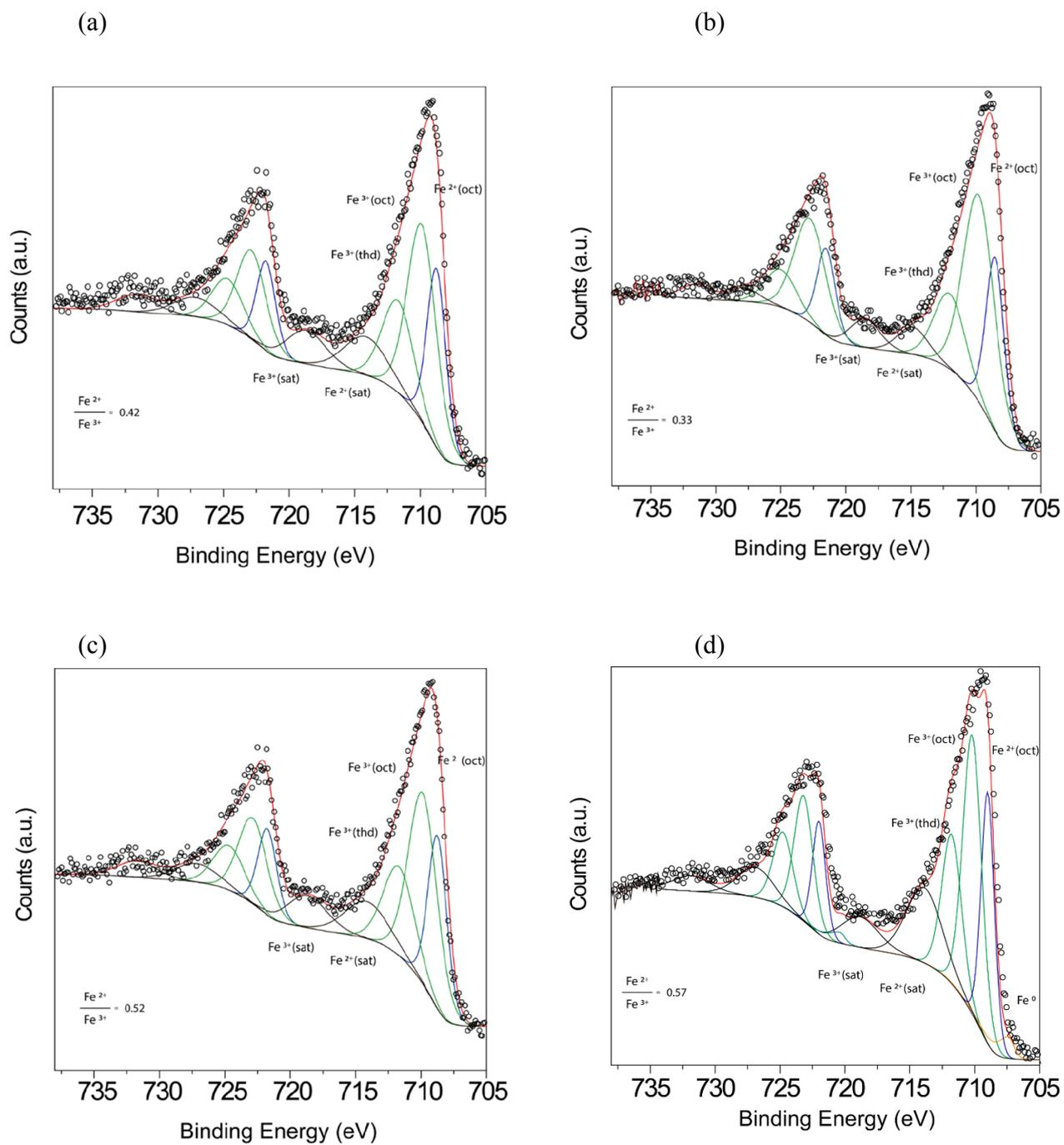
**Figure 2.** XPS spectrum for (a, c) FePc-CNT, (b, d) FePc-Py-CNT, (a, b) before, and (c, d) after exposition to O<sub>2</sub>.
