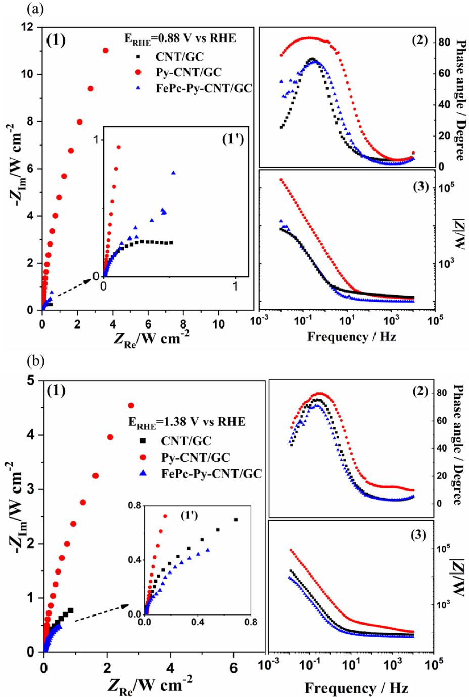
**Figure 5.** (a-1) Nyquist plots at 0.88 V vs. RHE, (a-2, a-3) Bode plots for CNT/GC, Py-CNT/GC and FePc-Py-CNT/GC under  $\text{N}_2$  and  $\text{O}_2$  atmosphere in 0.1M KOH for ORR. (b-1) Nyquist plots at 1.38 V vs. RHE, (b-2, b-3) Bode plots for CNT/GC, Py-CNT/GC and FePc-Py-CNT/GC under  $\text{N}_2$  and  $\text{O}_2$  atmosphere in 0.1M KOH for OER.
