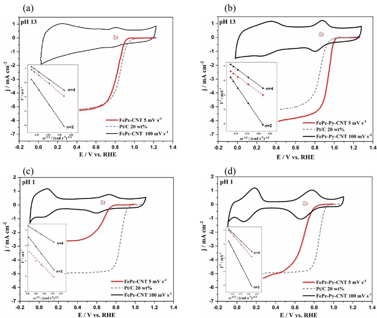
**Figure 3.** Cyclic Voltammetry at  $100\text{mV s}^{-1}$  in  $\text{N}_2$  and polarization curve at  $5\text{mV s}^{-1}$ , 1600 rpm and  $\text{O}_2$  saturated solution for (a, c) FePc-CNT, (b, d) FePc-Py-CNT, and (a-d) Pt/C 20wt% in (a, b) 0.1M KOH and (c, d) 0.1M H<sub>2</sub>SO<sub>4</sub> solution. (a-b) Inset show Koutecky-Levich plot determined at 0.35 and 0.45 V vs. RHE in acid and alkaline media, respectively.
