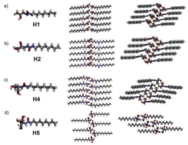
**Figure 2.** Crystal structures in stick representation of : a) **H1**, b) **H2**, c) **H4** and d) **H5** (N, blue; C, gray; O, red; H, white) showing (left) the monomeric molecules together with the lateral packing of H-bonded hydroxyl tetrads (middle) and their perpendicular packing *via* urea-urea and urea-hydroxyl H-bonding ribbons (right).
