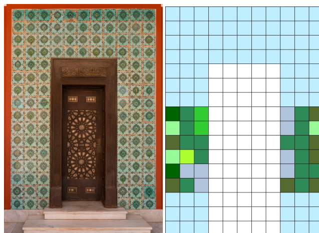
Figure 3: Left: Photo of one of the exterior door in the French Embassy, framed by Iznik ceramic tiles. Right: Clustering realized on these tiles by hyperspectral classification of pigments.
