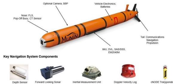
Fig. 2. The Kongsberg Mumin 1500 AUV and its components
