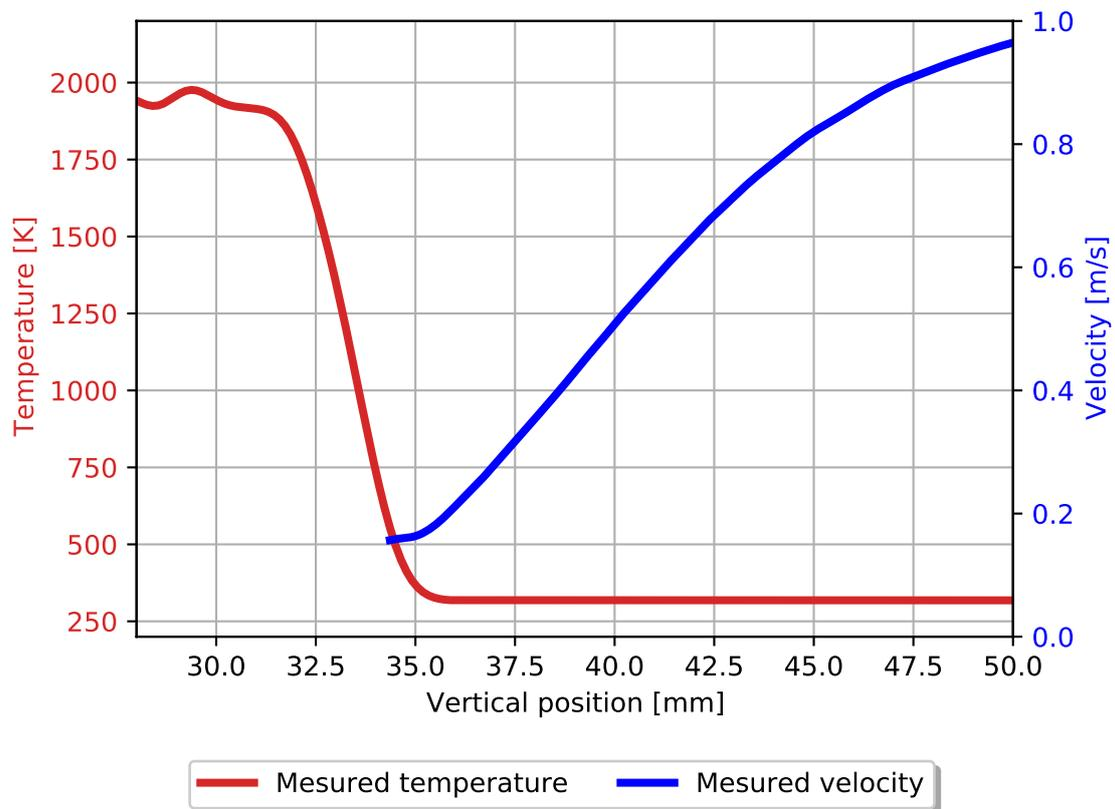
Fig. 8: Velocity and temperature along the burner axis.
