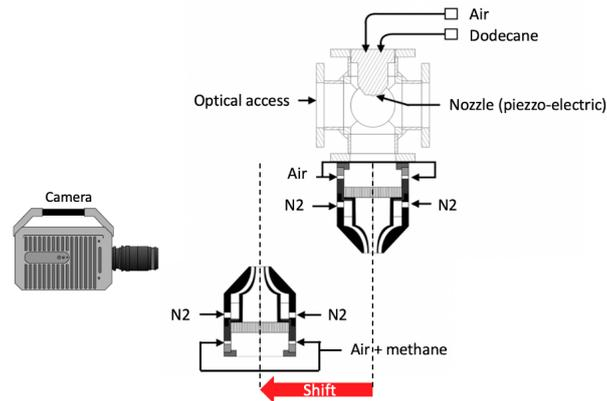
Fig. 13: Scheme of the offset burner configuration.
