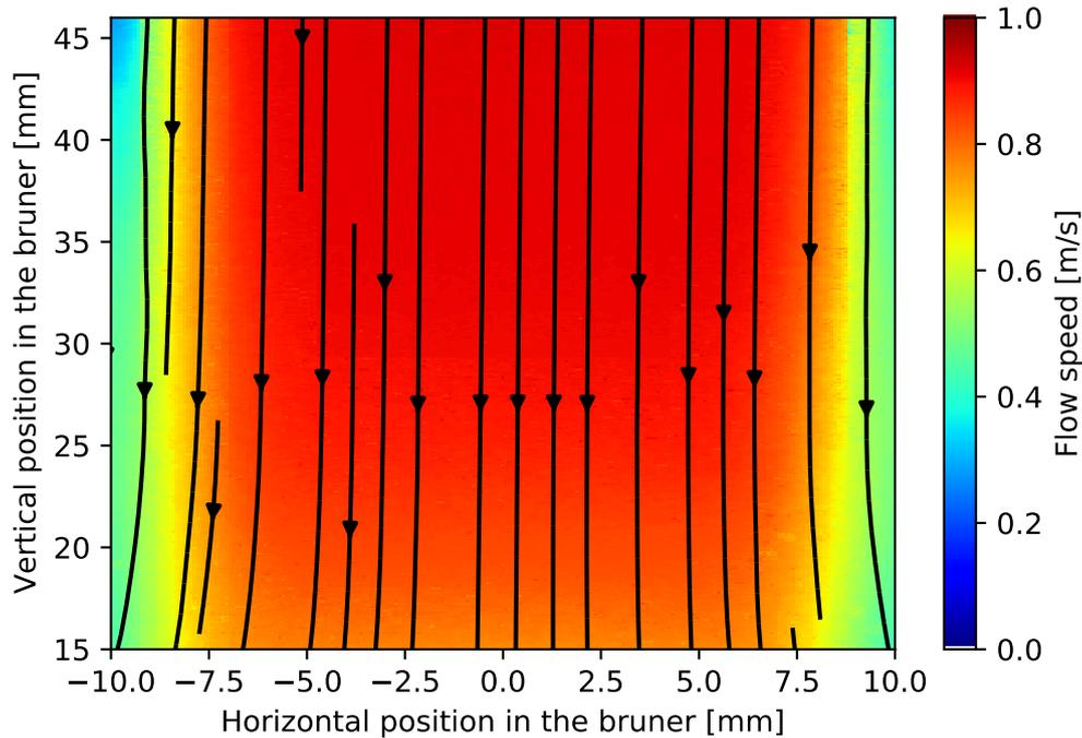
Fig. 12: Velocity map for the offset burner configuration.
