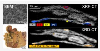
collection. For each fragment, the carbon-black pigment found in the ink is identified as flame carbon (lampblack or soot). Using X-ray diffraction computed tomography, we show that the diffraction signal of the carbon-based pigment itself can be isolated. As a result, a contrast with the papyrus support is obtained, even in the absence of a specific chemical element in the ink. This is opening up new opportunities to decipher words written millennia ago, as part of our Cultural Heritage.
