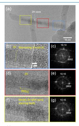
Figure 8. (a) HRTEM image of a SiNW with mostly the 2H phase; (b) alternating 2H and 3C domains at the bottom of the NW; (d) 2H phase in the middle; and (f) 2H phase with stacking faults at the top. The corresponding FFT images of (b,d,f) are shown in (c,e,g), respectively. Scale in (b) is for (b,d,f).
