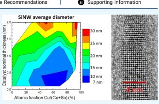
transmission electron microscopy analysis shows that both 3C and 2H polytypes are present, with the 2H hexagonal diamond structure appearing in 5-13% of the analyzed NWs per sample.
