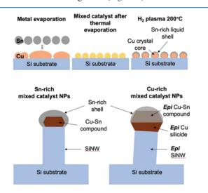
**Figure 5.** Schematic diagram of bimetallic Cu–Sn catalyst evolution at various stages of the SiNW growth process. The two figures at the bottom highlight the case of a NW growth led by a Sn-rich mixed catalyst NP (left) and a Cu-rich mixed catalyst NP (right).
