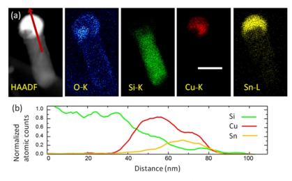
**Figure 4.** EDX mapping analysis of a SiNW synthesized with the majority Cu catalyst (1 nm Sn/0.8 nm Cu, 65 at. % Cu). (a) HAADF image and maps of the elements, scale bar = 50 nm; the contrasts of O-K and Sn-L images have been enhanced, compared to Si-K and Cu-K, for the sake of visibility. (b) Normalized atomic profiles of Si, Cu, and Sn along the red arrow in (a). Note the segregation between Sn and Cu in the catalyst.
