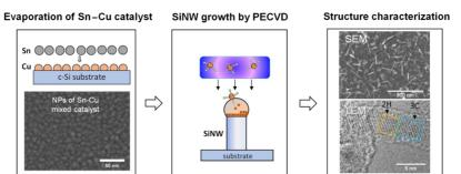
**Figure 1.** Schematic of the experiments reported. SiNWs were grown by PECVD with catalysts made of different amounts of Cu and Sn deposited sequentially (21 compositions in total, as shown in Figure 6; see Supporting Information, Table S1). The structure of the deposit, of the NWs, and of the catalysts was studied by SEM and TEM (see details in the Experimental Section).
