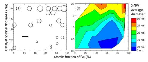
**Figure 6.** SiNW average diameter as a function of total nominal thickness (Y axis) and atomic fraction of Cu (X axis) in the multiphase catalyst. The SiNWs are grown on c-Si substrates and the average diameters of SiNWs are measured by SEM. (a) Plot showing the 21 data points; the size of the disks indicates the NW average diameter, scale bar = 30 nm. (b) Contour plot of the same data.
