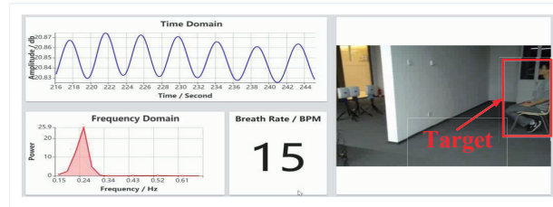
(b) Respiration sensing through wall
