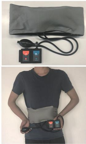
Fig. 16. Belt logger sensor.
