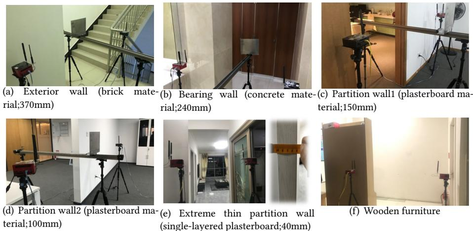
Fig. 7. Experimental environments with different types of walls.
