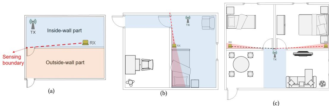
Fig. 25. (a) Space division when the wall is leveraged as a sensing boundary; (b) transceivers deployment for single-boundary determination: blue area for transmitter deployment and red area for receiver deployment; and (c) transceivers deployment for multiple-boundary determination: blue area for transmitter deployment and red area for receivers deployment.
