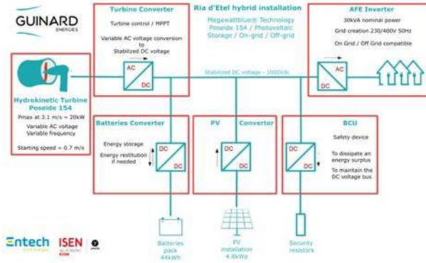
Fig. 2. Architecture synoptic of a Poseide P154 installation. ©Guinard Energies.
