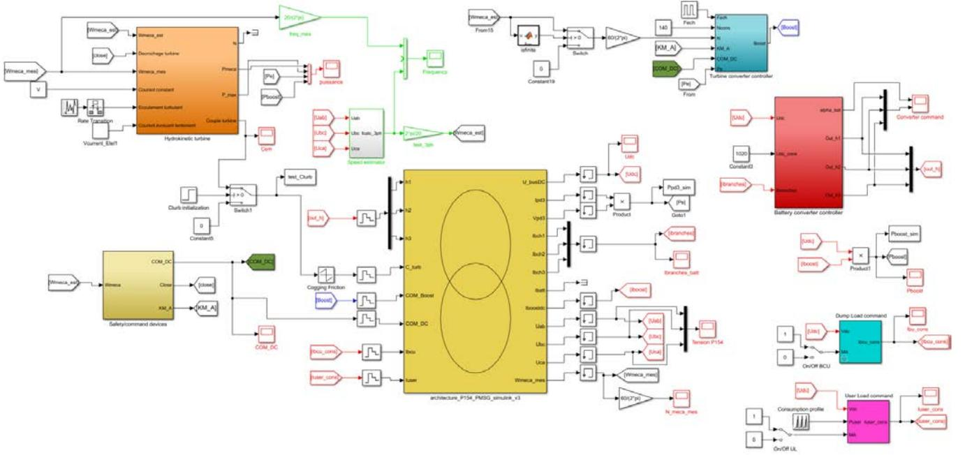
Fig. 4. Tidal stream turbine converter modeling with cosimulation.
