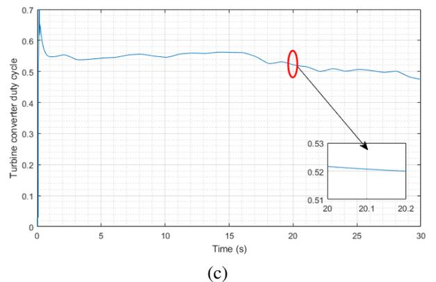
Fig. 9. Evolution of variables, Matlab/Simulink Instantaneous Modeling. (a)  $P_{elec}$ ,  $P_{turb\_conv}$ , (b)  $\Omega_{est}$ , (c)  $\alpha_{turb\_conv}$ .
