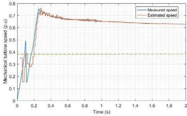
Fig. 7. Evolution of measured and estimated mechanical speed during a start.
