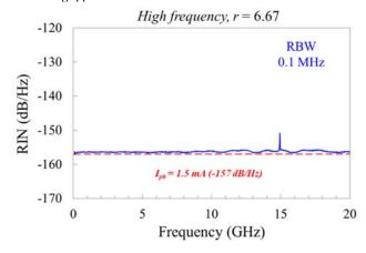
**Fig. 6.** High frequency RIN for 1.48 mA detected photocurrent (RBW = 0.1 MHz, sweep points 10001, sweep count 100). The pumping rate,  $r = I/I_{th}$ , is 6.67. Red dashed line is the relative shot-noise level for 1.48 mA detected photocurrent -157 dB/Hz.
