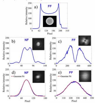
**Fig. 2.** Beam patterns imaged with a InGaAs camera. a) Far-field (FF) resonant amplified electroluminescence measured at a current density of 19.1 kA/cm². b) and c) Near-field (NF) and FF profiles of the laser beam obtained when the output mirror is positioned for maximum power extraction (60 mA pump current). d) and e) NF and FF profiles obtained for a slightly shorter cavity and exhibiting a  $TEM_{00}$  single transverse mode oscillation.
