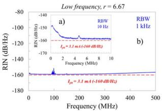
Fig. 5. RIN for 3.1 mA detected photocurrent (sweep points 10001, sweep count 100). The pumping rate, r = I/I<sub>th</sub>, is 6.67. Red dashed lines are the relative shot-noise level for 3.1 mA detected photocurrent (-160 dB/Hz). a) RIN at very low frequency with RBW = 10 Hz , b) RIN at low frequency with RBW = 1 kHz.
