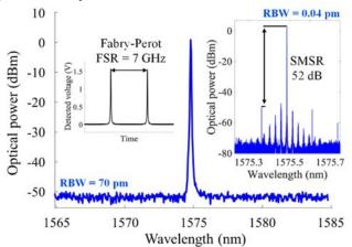
**Fig. 3.** Optical spectrum of the EP-QWs-VECSEL. Left hand-side inset: Fabry-Perot analysis testifying single frequency operation of the laser. Right hand-side inset: high resolution optical spectrum revealing the side mode suppression ratio of the laser.
