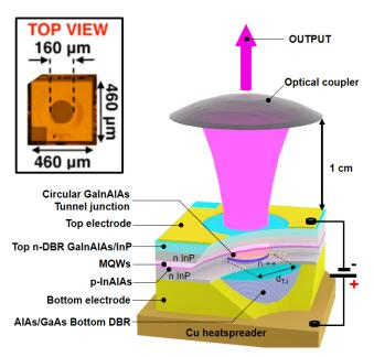
**Fig. 1.** Schematic of electrically pump VCSEL based quantum wells imbedded in an external high finesse cavity. MQWs: multiple quantum wells,  $d_{TI}$ : tunnel junction diameter, DBR: Distributed Bragg Reflector.
