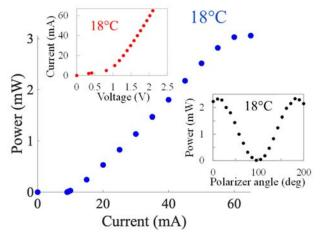
Fig. 4. The CW LI, IV characteristics and polarization state of the EP-QWs-VECSEL at  $18^{\circ}$ C.
