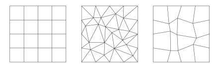
FIGURE 1. Coarsest Cartesian, distorted triangular, and distorted Cartesian meshes used in Section 5.
