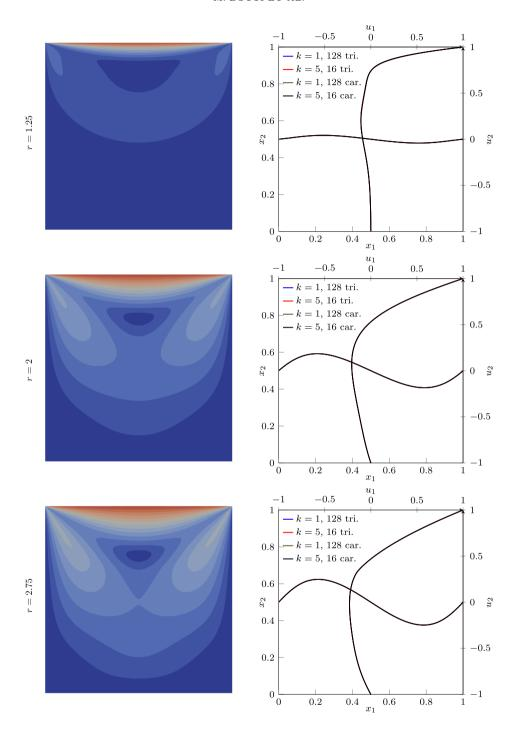
FIGURE 4. Numerical results for the test case of Section 5.2. Left: velocity magnitude contours (15 equispaced values in the range [0,1]). Computations on a Cartesian mesh of size  $128 \times 128$  with k=5. Right: horizontal component  $u_1$  of the velocity along the vertical centreline  $x_1=\frac{1}{2}$  and vertical component  $u_2$  of the velocity along the horizontal centreline  $x_2=\frac{1}{2}$ .
