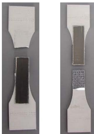
FIG. 4 – Rupture du patch composite.
