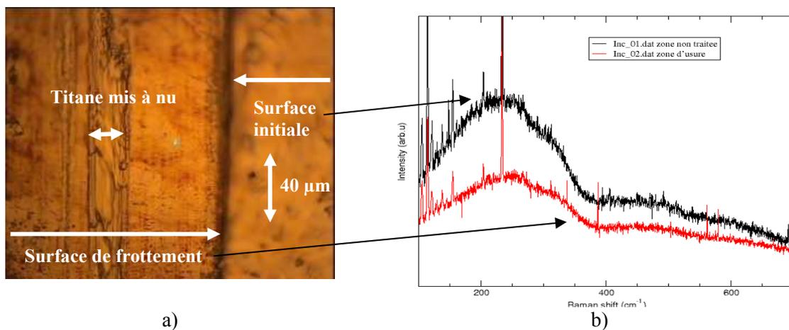
FIG. 3 - Couche incolore a) micrographie b) Spectres Raman
