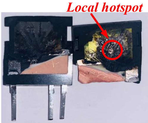
Fig. 6. Decapsulated device 1, 3kV IGBT (i4 pak), showing local hotspot failure.
