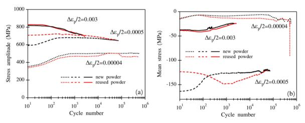
Figure 11 : Example of the evolution of stress amplitude and mean stress during fatigue tests for different stress amplitudes
