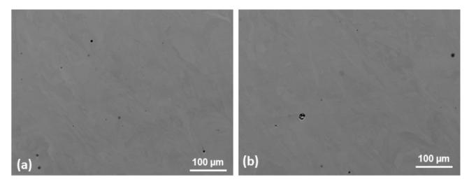
Figure 3: SEM images of polished R50 samples showing porosity in (a) horizontal section (XY) and vertical section (XZ).
