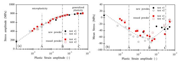
Figure 10: Comparison between the cyclic stress-strain curves of samples elaborated from new (R0-black) and reused (R50-red) powder. (a) Evolution of stress amplitude with plastic strain and b) evolution of mean stress with plastic strain. Vertical dashed lines correspond to strain amplitude selected for fatigue tests. Only two sample curves have been plotted for each kind of sample.
