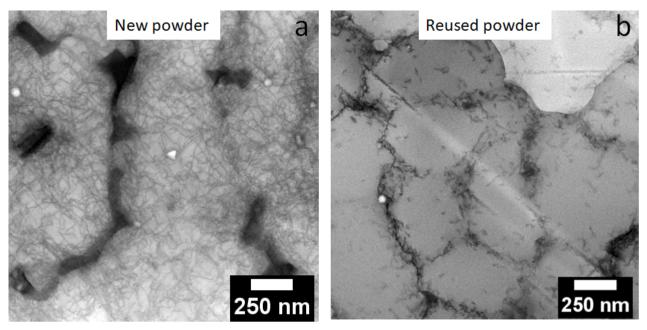
Figure 5: Bright field STEM images of new powder and reused powder made samples. Dislocation walls, Laves phases, carbides and Al2O3 particles are present in both samples.
