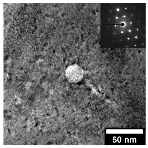
Figure 7 : Bright field TEM image showing Al2O3 particle and the associated SAED in new powder made sample. Matrix is close to [110] zone axis.
