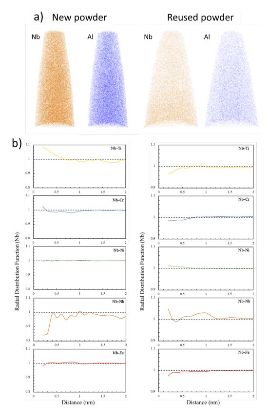
Figure 9: Reconstructed APT volumes from new (50\*50\*125nm3) and reused powder (50\*50\*84 nm3) made samples with b) corresponding Radial Distribution Functions (RDF) for Nb ions.
