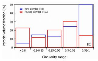
Figure 2: (a) Size distribution of powder particles for the new and reused powder with their corresponding circularity distribution in (b).
