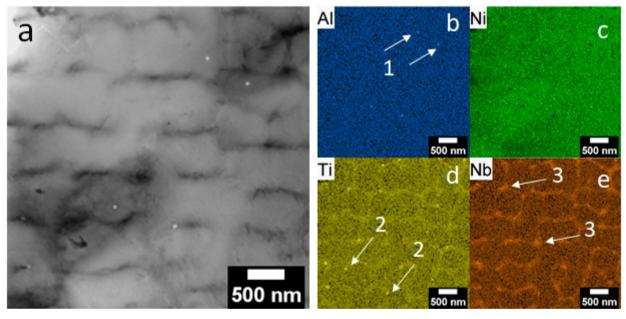
Figure 6: STEM bright field image (a) and EDX analysis (b-c-d-e) at low magnification of new powder sample (R0). Intercellular region is enriched in Nb and Ti. This analysis also emphasizes the presence of Al2O3 precipitates and Ti carbides.
