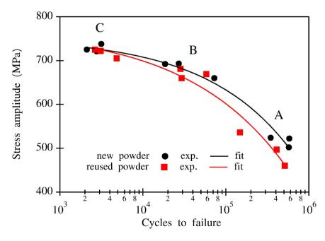
Figure 12 : Comparison of SN curves for samples elaborated from new (black) and reused (red) powder. Lines correspond to the fit.
