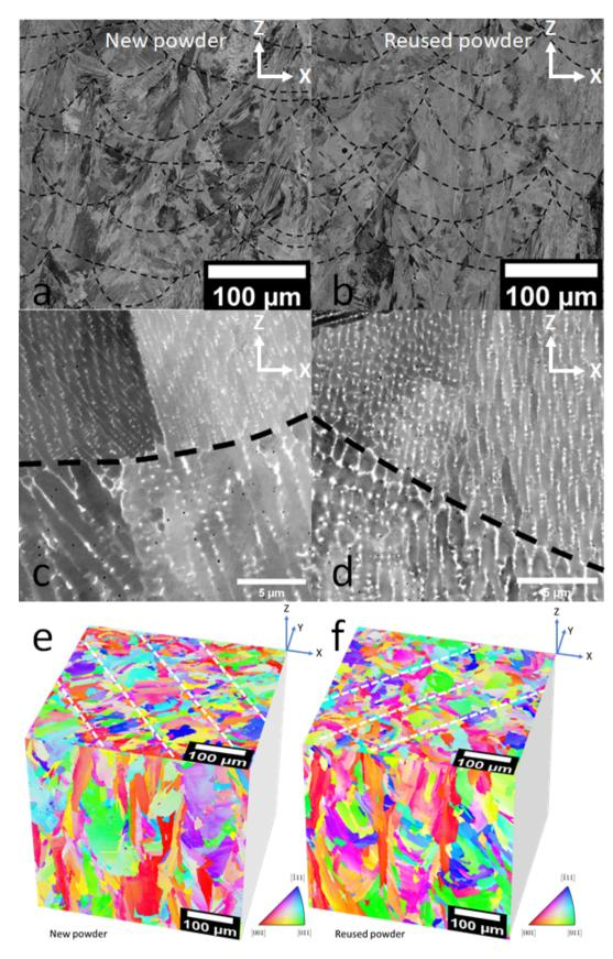
Figure 4: Backscattered electron images at low magnification (a-b) and high magnification (c-d) and IPF (along the building direction) maps (e-f). a-c-e are related to samples manufactured with the new powder and b-d-f with the 50 times reused one. Black dashed lines in a-b-c-d are MPB. White dashed lines in e-f delimit small and big grains in xy planes.
