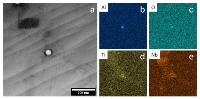
Figure 8 : STEM bright field image (a) of new powder made sample and associated EDX element maps (b-c-d-e) showing an Al2O3 particle surrounded by a shell enriched in Ti and Nb.
