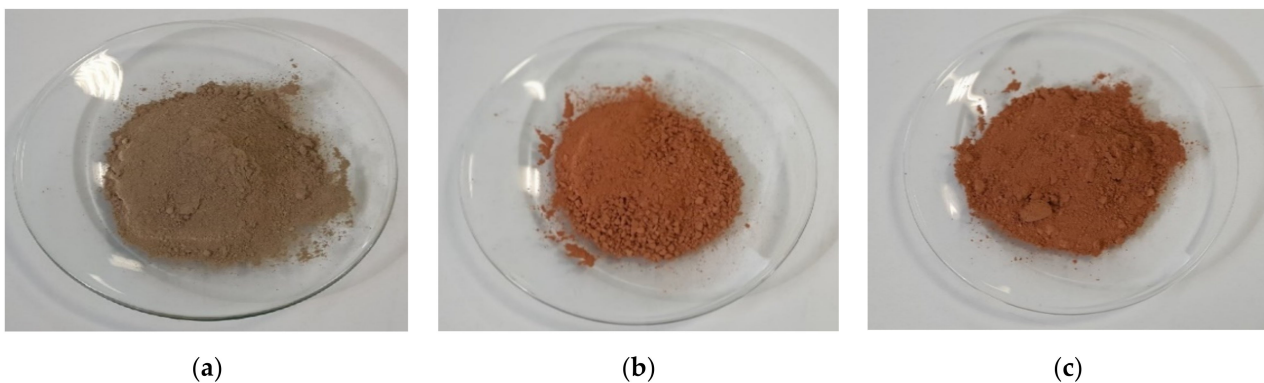
Figure 4. Visual aspect of (a) raw dried; (b) calcined and (c) crushed calcined sediment.
