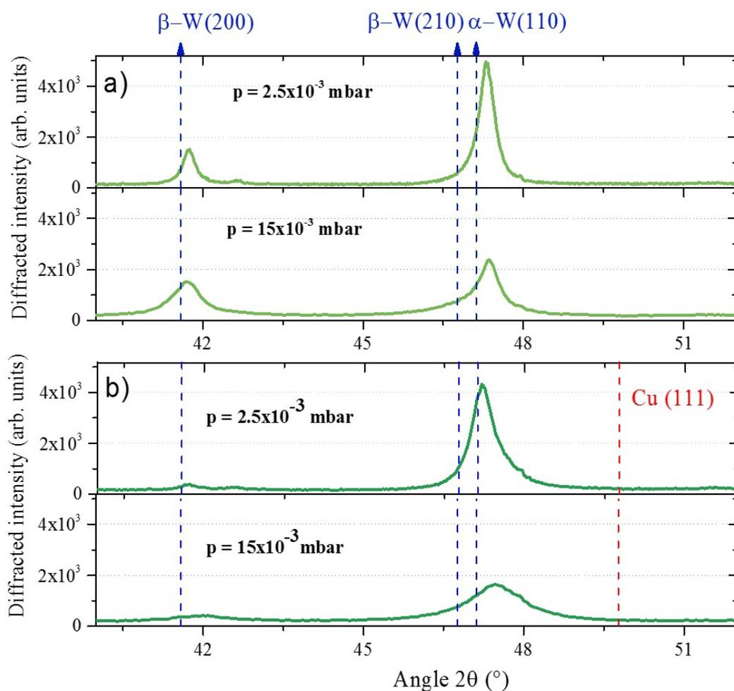
Figure 6: (a) XRD patterns of 1000 nm thick W thin films sputter-deposited on (100) Si substrate with an angle  $\alpha = 80^\circ$ , and for an argon sputtering pressure of  $2.5 \times 10^{-3}$  and  $15 \times 10^{-3}$  mbar. (b) XRD patterns of 1000 nm thick W-
