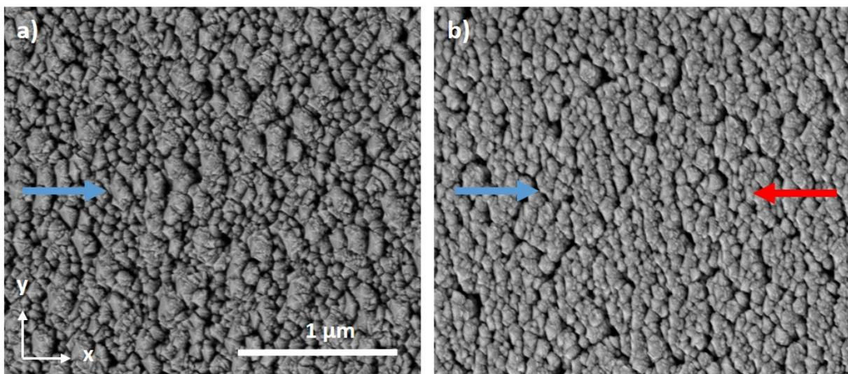
Figure 5: SEM images of: (a) the surface of the W film and (b) the surface of the W-Cu film both deposited at high sputtering pressure ( $15 \times 10^{-3}$  mbar) with a thickness of 1000 nm. Blue and red arrows indicate the direction of incoming W and Cu particle fluxes, respectively.
