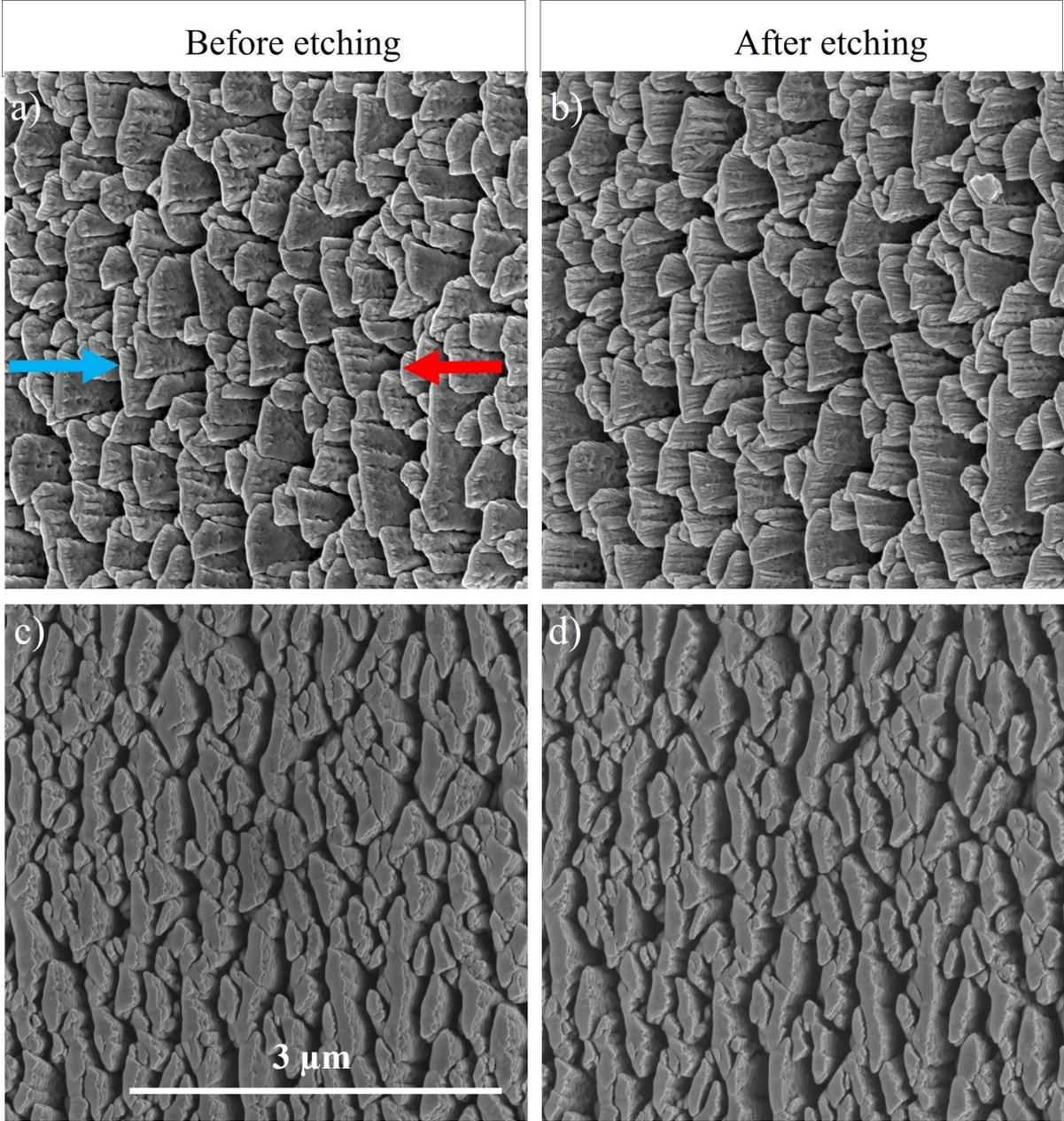
Figure 7: SEM images of the surface of a W-Cu film 1000 nm thick viewed at the same location: a) before and b) after Cu etching, and with a 45° tilt angle of observation: c) before and d) after Cu etching. Blue and red arrows indicate the direction of incoming W and Cu particle fluxes, respectively.
