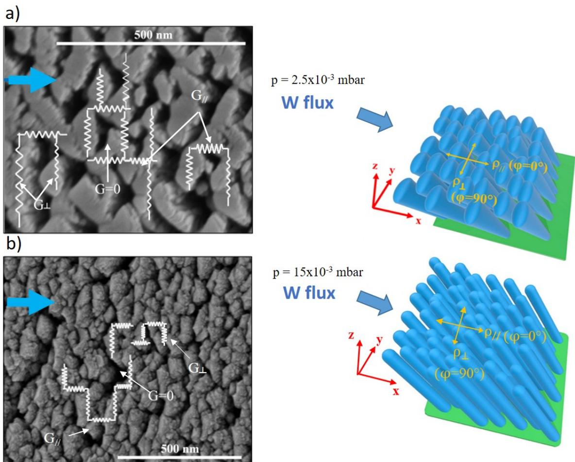
Figure 2: Schematic representation of the variation of conductance directions in the film with SEM observations of two W films 1000 nm thick deposited at: a)  $2.5 \times 10^{-3}$  mbar and b)  $15 \times 10^{-3}$  mbar. Blue arrows indicate the incoming flux of W atoms.
