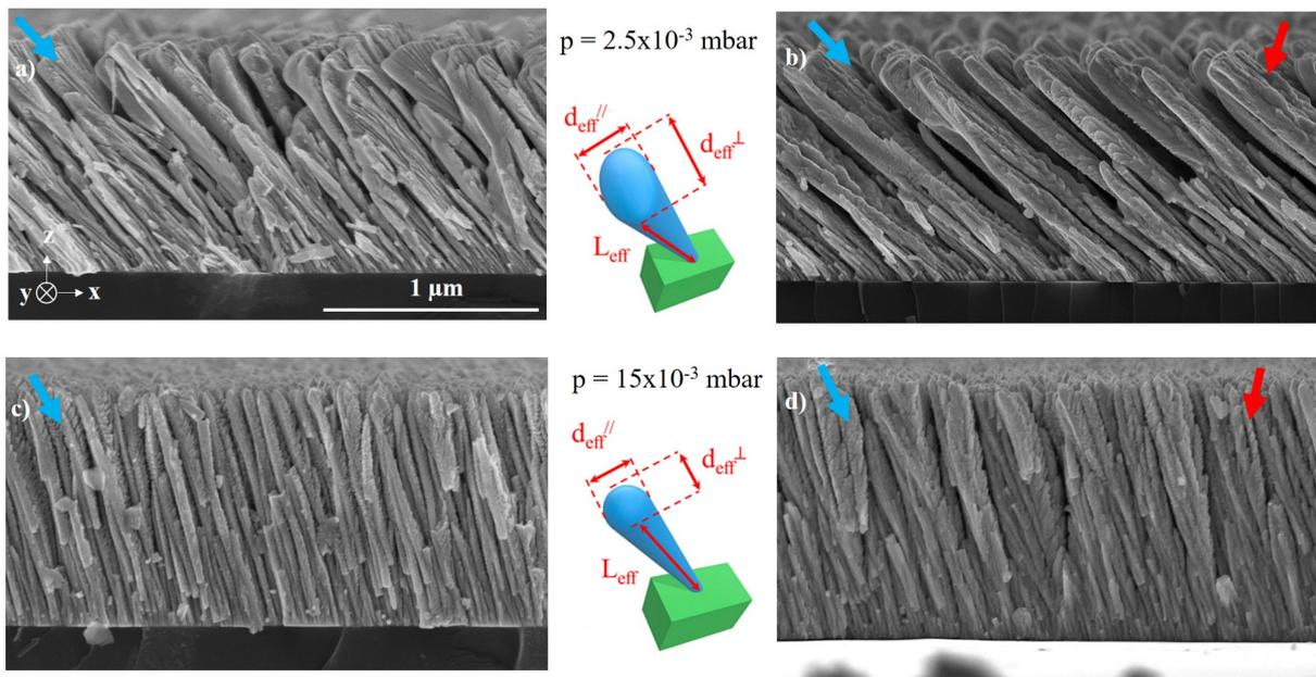
Figure 3: Schematic representation of the variation of effective widths and effective length. Cross-section observations by SEM of W and W-Cu films 1000 nm thick deposited at: a) and c)  $2.5 \times 10^{-3}$  mbar, and b) and d)  $15 \times 10^{-3}$  mbar. Blue and red arrows indicate the direction of incoming W and Cu particle fluxes, respectively.
