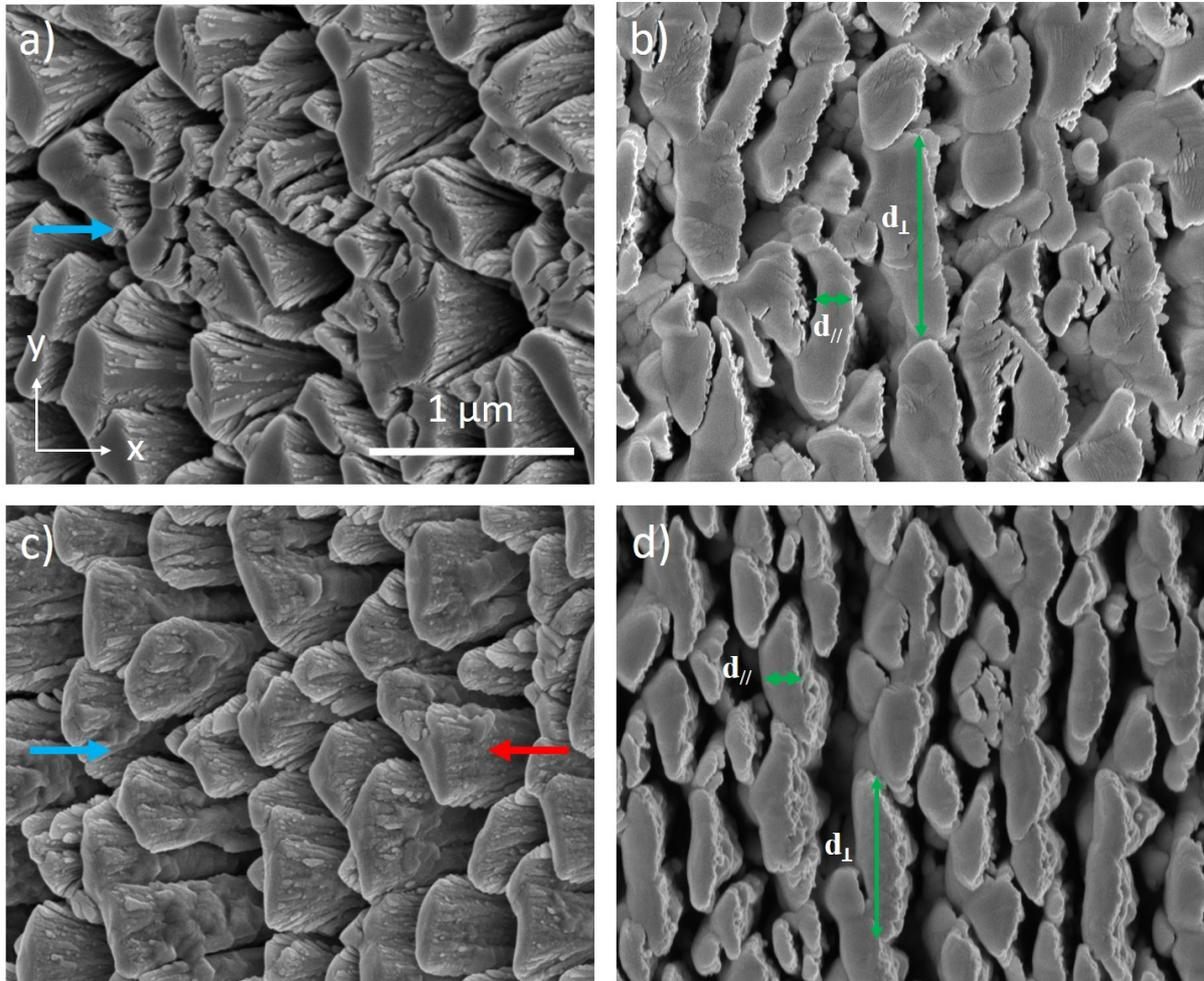
Figure 4: SEM observations of: (a) the surface of W film 1000 nm thick sputter-deposited at  $2.5 \times 10^{-3}$  mbar; (b) the same surface after a tilt of  $35^\circ$ ; (c) the surface of a W-Cu film 1000 nm thick; (d) the same surface after a tilt of  $45^\circ$ . Blue and red arrows indicate the direction of incoming W and Cu particle fluxes, respectively.
