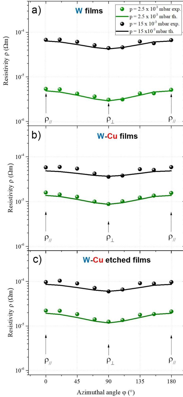
Figure 8: Variation of electrical resistivity measured at room temperature (300 K) as a function of azimuthal angle  $\varphi$  for: a) W films, b) W-Cu films and c) etched W-Cu films 1000 nm thick sputter-deposited at  $2.5 \times 10^{-3}$  and  $15 \times 10^{-3}$  mbar.  $\rho_{//}$  et  $\rho_{\perp}$  represent resistivity in the direction parallel and perpendicular to W and Cu fluxes,
