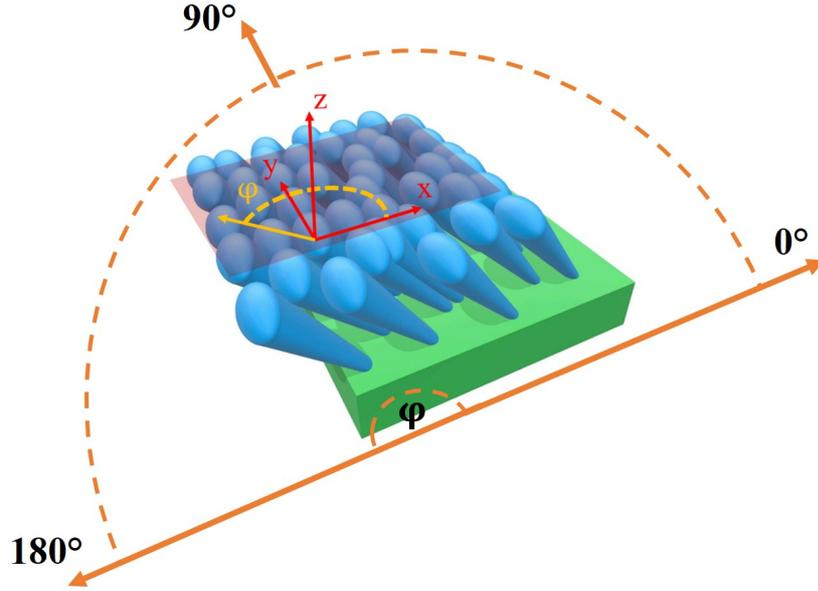
Figure 1: Schematic representation illustrating the film orientation used for resistivity measurements as a function of the azimuthal angle  $\varphi$ .
