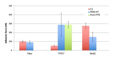
619Figure 9 – Mean adhesion force and associated standard deviation (black lines) for each component620of pure PTFE, PGM-HT and AAC-C1
