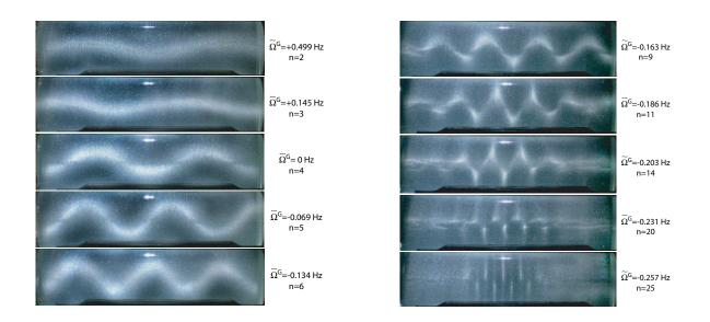
Figure 2: Variation of the wavelength of the elliptical instability versus the global rotation  $\tilde{\Omega}^G$  for a given cylinder of radius  $\tilde{R} = 2.75$ cm and height  $\tilde{H} = 21.4$ cm with an eccentricity  $\varepsilon = 0.085$  rotating at  $\tilde{\Omega}^F = 0.505 \pm 0.005$ Hz (Re =  $2.40 \times 10^3$ ). In these pictures, the rotation axis is horizontal.
