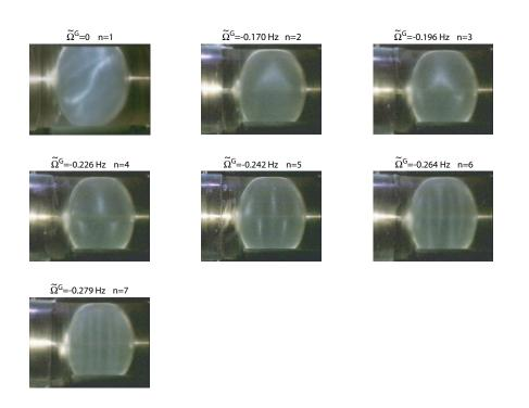
Figure 3: Pictures of the flow structure associated with the elliptical instability for different global rotation rates  $\tilde{\Omega}^G$  in the deformed sphere with an eccentricity  $\varepsilon = 0.20$  and a fixed fluid rotation  $\tilde{\Omega}^F = 0.500 \pm 0.005$ Hz (Re =  $1.49 \times 10^3$ ). The measured number n of axial half-wavelengths is also indicated. In these pictures, the rotation axis is horizontal.
