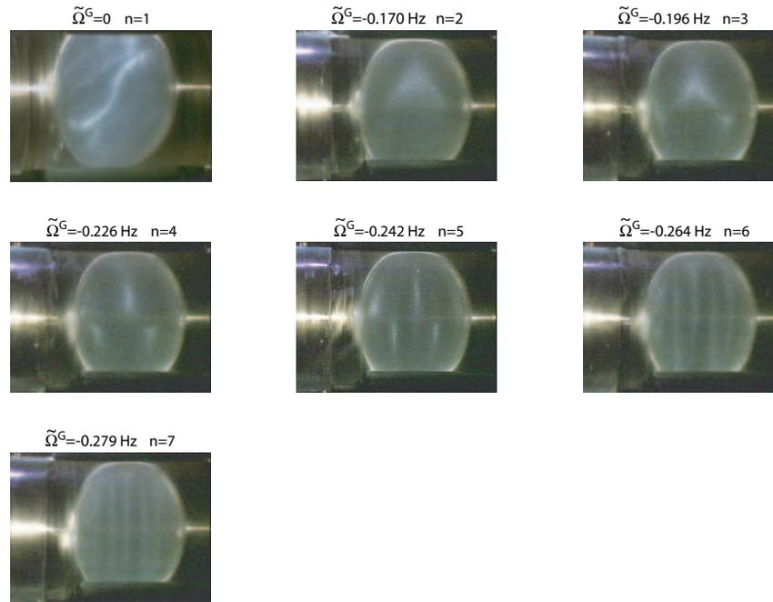
Figure 3: Pictures of the fbw structure associated with the elliptical instability for different global rotation rates  $\tilde{\Omega}^G$  in the deformed sphere with an eccentricity  $\varepsilon = 0.20$  and a fixed fluid rotation  $\tilde{\Omega}^F = 0.500 \pm 0.005 \text{ Hz}$  ( $\text{Re} = 1.49 \times 10^3$ ). The measured number  $n$  of axial half-wavelengths is also indicated. In these pictures, the rotation axis is horizontal.
