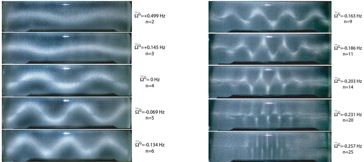
Figure 2: Variation of the wavelength of the elliptical instability versus the global rotation  $\tilde{\Omega}^G$  for a given cylinder of radius  $\tilde{R} = 2.75\text{cm}$  and height  $\tilde{H} = 21.4\text{cm}$  with an eccentricity  $\varepsilon = 0.085$  rotating at  $\tilde{\Omega}^F = 0.505 \pm 0.005\text{Hz}$  ( $\text{Re} = 2.40 \times 10^3$ ). In these pictures, the rotation axis is horizontal.
