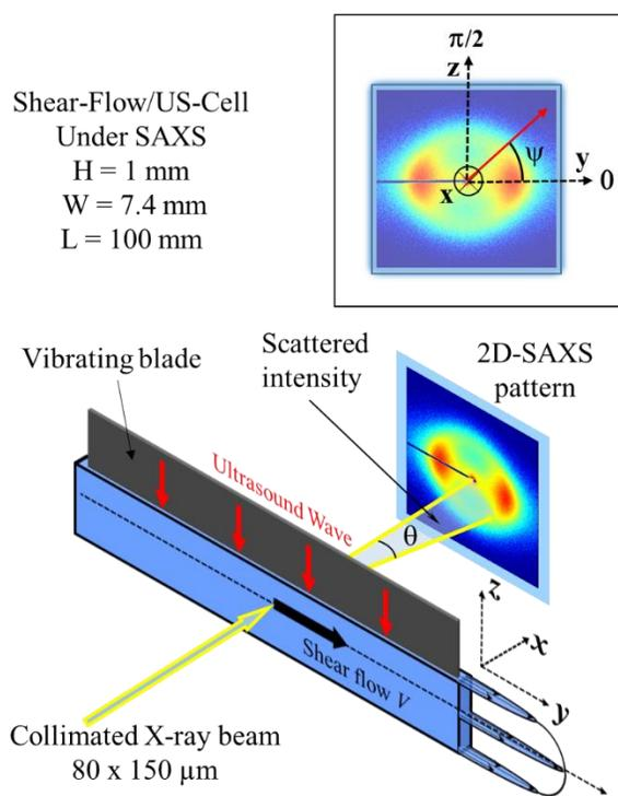
**Figure 1. Schematic description of the SAXS experiment with the dedicated Shear flow/US-Cell used to monitor the time dependent changes of structural organization under simultaneously applied shear flow (horizontal stress force) and ultrasound waves (vertical acoustic radiation force).**
