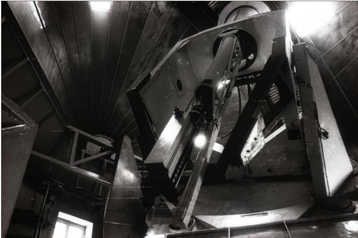
Figure 18: The 0.15-m coronagraph with its spectrograph at the back, mounted in the fork of the Pic du Midi Turret-Dome (1966), after removal of the 0.38-m refractor (courtesy: OCA).
