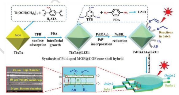
Photocatalytic tandem reaction in a dual-chamber microreactor
