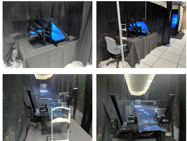
Figure 3: View of physical display hardware at Location A for running experiments on binocular accommodation and vergence overdriving as described in Section 3.
