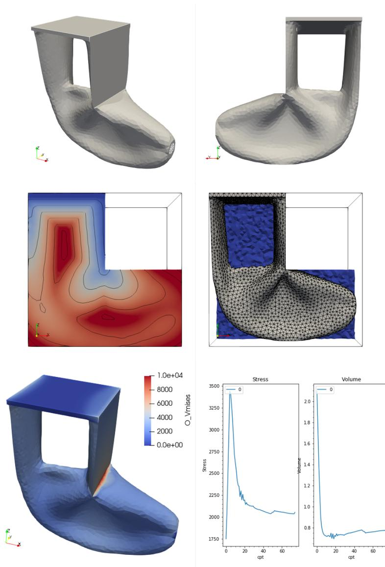
**Fig. 3** Two views of the optimized design with  $\alpha = 2$  (top). Level set function and body-fitted mesh of the optimized design (middle). Von Mises stress and convergence history for the L-beam test case with  $\alpha = 2$  (bottom).
