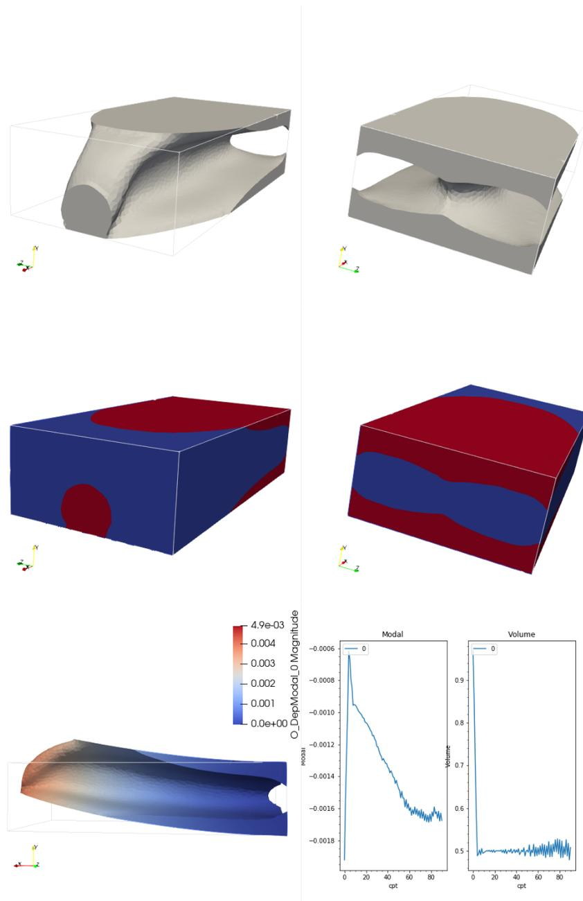
**Fig. 6** Two views of the optimized design (top). Optimized design inside the design space. First eigenmode amplified by a factor of 70 and convergence history for the test case described in Section 7.2 (bottom).
