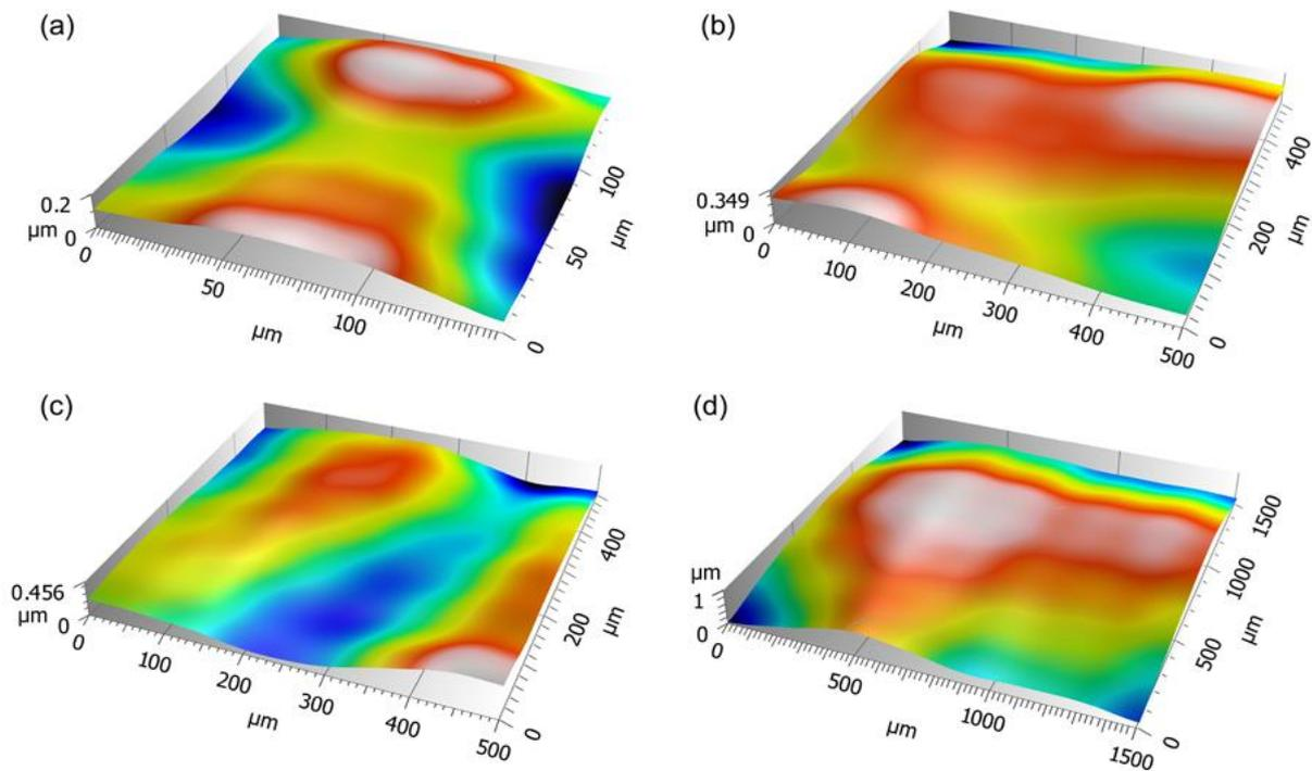
Figure 5: Examples of waviness computed for each specimen.
