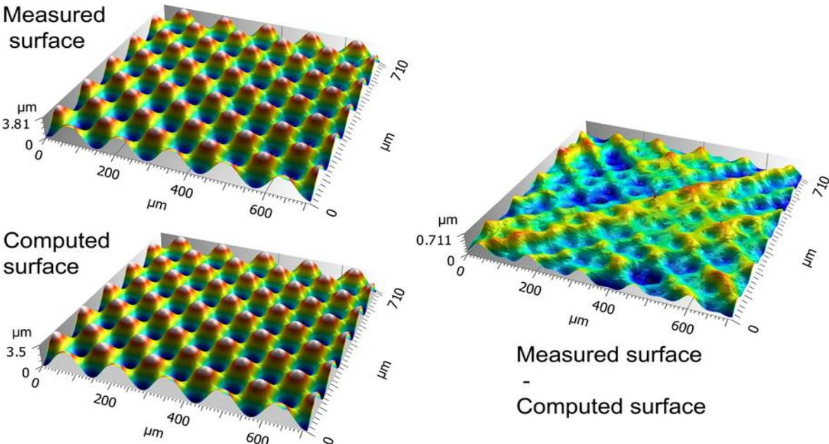
Figure 7: Example of measured surface for 10\_03, of the computed surface obtained with the identification of the parameters and of the surface obtained with the subtraction of the computed surface from the measured surface.
