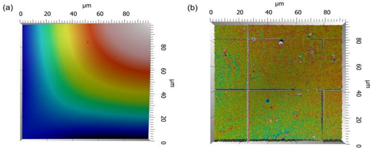
Figure 3: (a) Extraction of an area  $100\ \mu\text{m} \times 100\ \mu\text{m}$  from a measurement of 300\_30 and (b) corresponding area filtered with a high-pass Gaussian filter with a cut-off of  $3\ \mu\text{m}$ .
