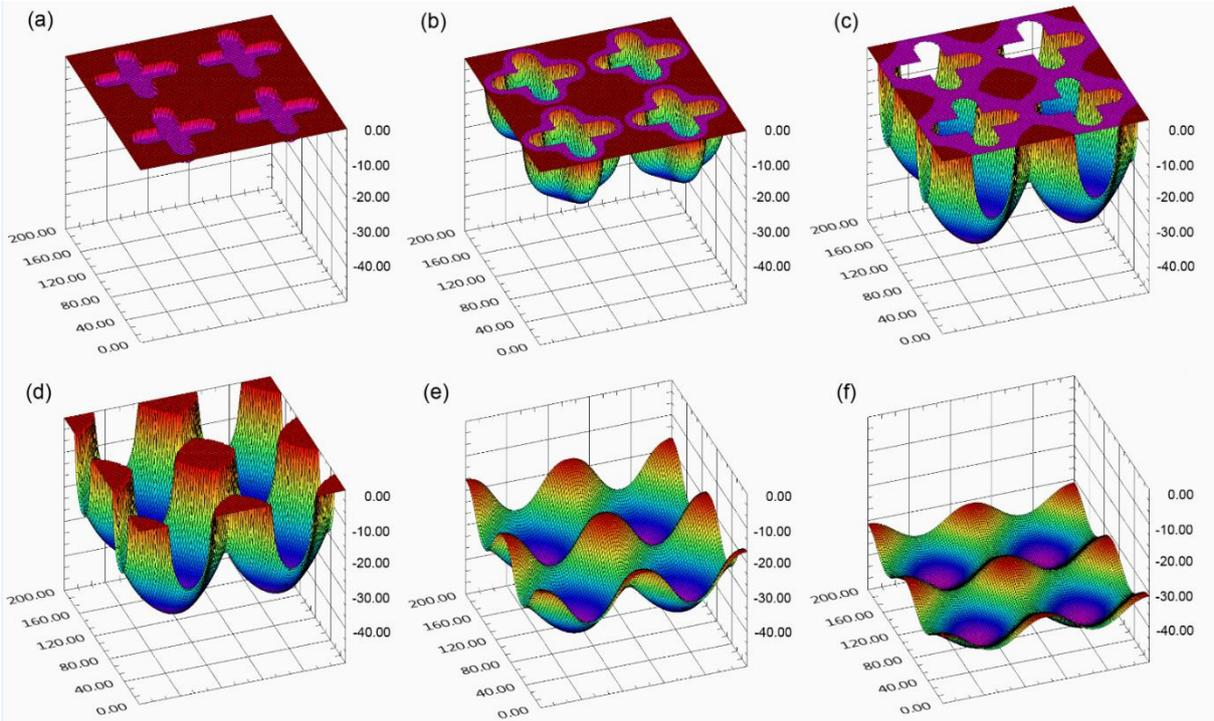
Figure 1 : Images extracted from the simulated two-step process used to obtain sinusoidal surfaces having an amplitude of 10  $\mu\text{m}$  and a period of 100  $\mu\text{m}$ : (a) to (c) preform creation through mask electrochemical micromachining, (d) to (f) mass transport limited dissolution of preforms after mask removal.
