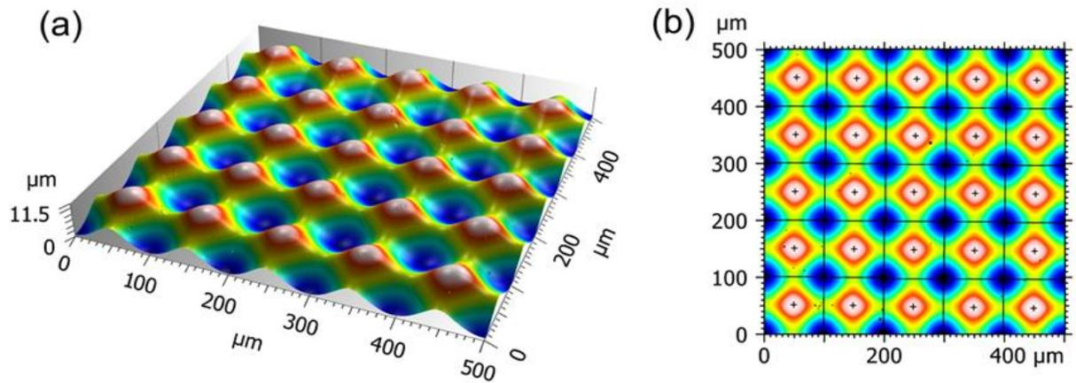
Figure 6 : (a) Example of a measurement of 100\_10 containing 5x5 periods and (b) the decomposition of this measurement into motifs using the watershed algorithm.
