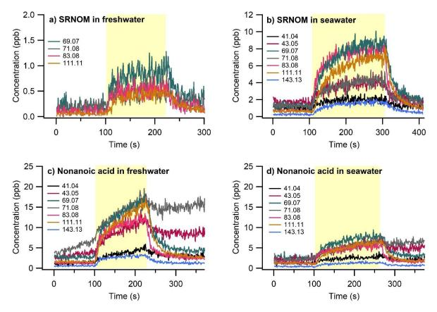
Figure 2: Select time traces for (a)  $10 \text{ mgL}^{-1}$  SRNOM only in freshwater, (b)  $10 \text{ mgL}^{-1}$ SRNOM only in seawater, (c) 2 mM nonanoic acid only in freshwater, and (d) 2 mM nonanoic acid only in seawater. All four experiments were run under air. In each case, the highlighted yellow region indicates the time during which the sample was illuminated during the experiment.
