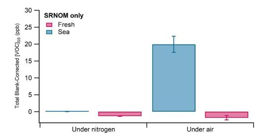
Figure 3: The total blank-corrected steady state concentrations (A-values) pulled from the kinetic growth fitting are shown for SRNOM only in freshwater (red) and seawater (blue). The experiments under nitrogen are shown on the left and the experiments under air are shown on the right. The error bars represent the error propagation of the standard deviation from the fitted equation.
