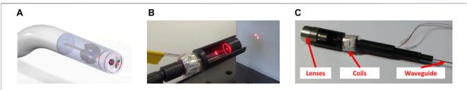
FIGURE 4 | Magnetically actuated laser scanners for endoscopic microsurgery. (A) Concept (B) Prototype based on a standard silicon optical fiber (Acemoglu et al., 2019). (C) Prototype based on a CO<sub>2</sub> laser waveguide (Acemoglu and Mattos, 2018).
