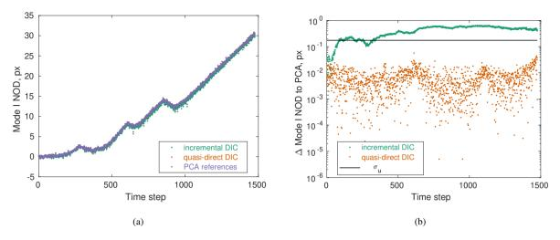
**Figure 21:** (a) Mode I NOD for the fourth 600°C case (MZ5-S1450G). (b) Absolute difference of mode I NOD using PCA references and the otehr cases
