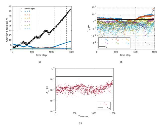
**Figure 20:** (a) Normalized RMS residuals for the fourth WST at 600°C (MZ5-S1450G) using PCA-based references  $\varphi^1$ . The four reference updated in quasi-direct DIC are shown in vertical dashed lines. (b) RMS difference between displacements for each tested truncation (Algorithm 1) and (c) for the proposed brightness correction (Algorithm 2). The standard displacement uncertainty  $\sigma_u$  is shown in solid black line.
