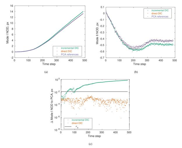
**Figure 9:** (a) Mode I and (b) mode II NODs for the room temperature WST (MZ1-S1450G). (c) Absolute difference of mode I NODs using PCA references and the other cases. The black solid line corresponds to the standard displacement uncertainty  $\sigma_u$ . Note that the results for PCA references appear to coincide with those of direct DIC in sub-figures (a) and (b). Their differences, shown in sub-figure (c) for mode I NOD, are very small compared to their magnitude.
