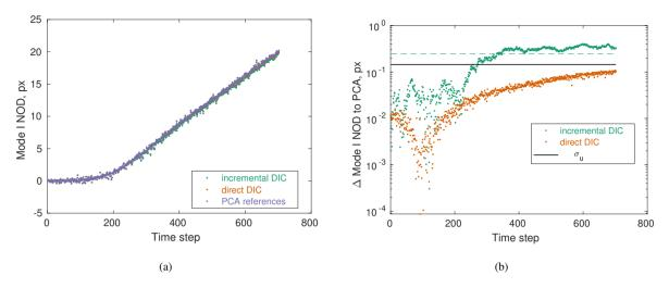
**Figure 12:** (a) Mode I NOD for the first WST at 600°C (MZ2-S1400). (b) Absolute difference of mode I NOD using PCA references and the other cases
