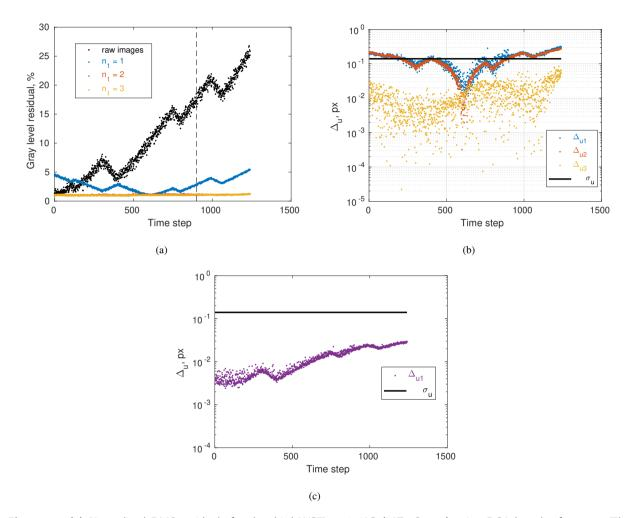
**Figure 17:** (a) Normalized RMS residuals for the third WST at 600°C (MZ4-S1450) using PCA-based references. The reference update for quasi-direct DIC is depicted with a dashed vertical line. (b) RMS difference between displacements for each tested truncation (Algorithm 1) and (c) for the proposed brightness correction (Algorithm 2). The standard displacement uncertainty  $\sigma_u$  is shown in solid black line
