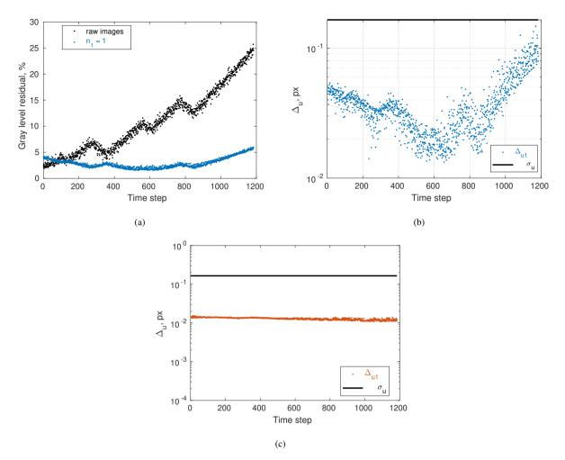
Figure 14: (a) Normalized RMS residuals for the second WST at 600°C (MZ3-S1400G) using PCA-based references  $\varphi^1$ . (b) RMS difference between displacements for each tested truncation (Algorithm 1) and (c) for the proposed PCA correction (Algorithm 2). The standard displacement uncertainty  $\sigma_u$  is shown in solid black line
