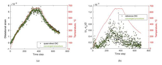
**Figure 24:** (a) Dilatational strain vs. time for DIC analyses with no brightness correction and for the last case after convergence. (b) Corresponding half difference of eigen strains. The temperature signals are shown in red
