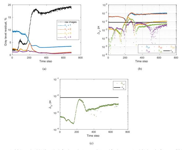
**Figure 23:** (a) Normalized RMS residuals for the preliminary analysis and for the case using PCA-based references. (b) RMS difference between displacement for each tested truncation (Algorithm 1). (c) RMS displacement difference for the first step of Algorithm 2. The standard displacement uncertainty  $\sigma_u$  is shown with a solid black line
