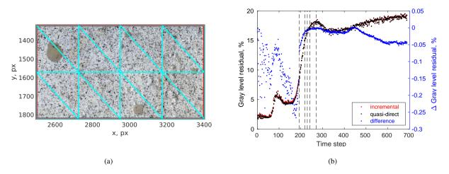
Figure 4: (a) Coarse mesh for the first kinematic correction. (b) Normalized RMS gray level residual for the preliminary DIC step with incremental and quasi-direct approaches. The vertical dashed lines depict updates of reference images for quasi-direct DIC
