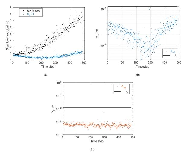
**Figure 8**: (a) Normalized RMS residuals for the room temperature WST (MZ1-S1450G) using PCA-based references  $\varphi^1$ . (b) RMS difference between displacements for each tested truncation (Algorithm 1) and (c) for the proposed PCA correction (Algorithm 2).  $\sigma_u$  is shown in solid black line
