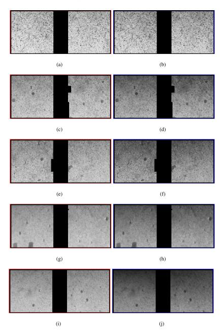
**Figure 6:** First (left column) and last (right column) images (ROIs for NOD calculations) in the  $\tilde{g}$  stacks for the room temperature experiment: MZ1-S1450G (a,b), and for the 600°C experiments: MZ2-S1400 (c,d), MZ3-S1400G (e,f), MZ4-S1450 (g,h), and MZ5-S1450G (i,j)
