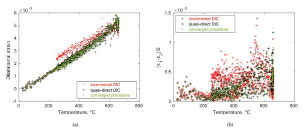
**Figure 25:** Dilatometry results showing the dilatational strain (a) and the half-difference between both eigen strains (b) as functions of temperature.
