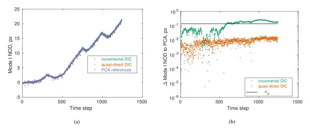
**Figure 18:** (a) Mode I NOD for the third 600°C test (MZ4-S1450). (b) Absolute difference of mode I NOD using PCA references and the other cases
