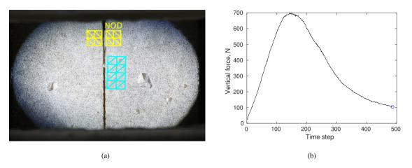
**Figure 5:** (a) Reference image for the room temperature WST (MZ1-S1450G). The yellow meshes depict the ROIs for NOD calculations. The sample is the same as that tested post-mortem in the dilatometry experiment (Figure 2), and the corresponding mesh is shown in cyan. (b) Applied force vs. time steps of image acquisitions. The blue circle depicts the final unloading level used for the evaluation of the work of fracture (and the end of the present analyses)
