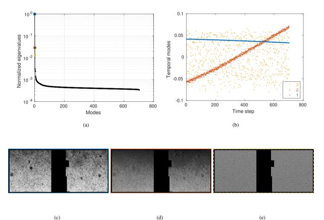
**Figure 10:** (a) Normalized eigenvalues of SVD of  $\tilde{g}$  for the first WST at 600°C (MZ2-S1400). (b) First three temporal modes and (c-e) corresponding spatial modes of the two ROIs used for NOD measurements (Figure 5)
