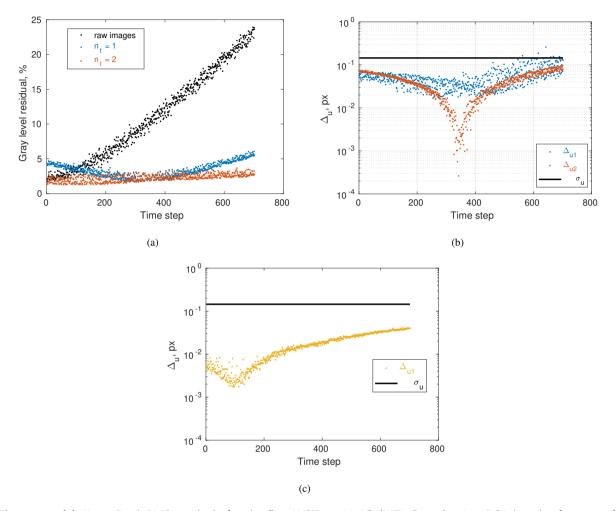
Figure 11: (a) Normalized RMS residuals for the first WST at 600°C (MZ2-S1400) using PCA-based references  $\varphi^1$ . (b) RMS difference between displacements for each tested truncation (Algorithm 1) and (c) for the proposed brightness correction (Algorithm 2). The standard displacement uncertainty  $\sigma_u$  in solid black line
