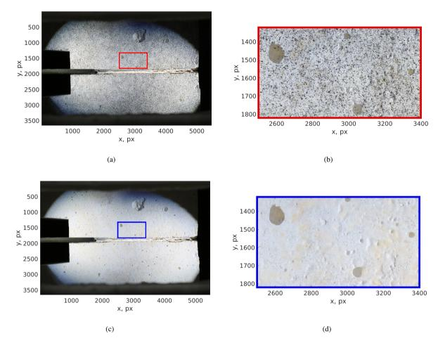
**Figure 2:** (a) Reference image prior to heating sample MZ1-S1450G (after the WST was performed). The ROI (red rectangle) is shown in sub-figure (b). (c) Last image after cooling down. The corresponding ROI (blue rectangle) is shown in sub-figure (d). Note that the speckle pattern almost disappeared during heating
