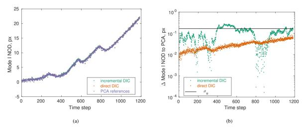
**Figure 15:** (a) Mode I NOD for the second 600°C WST (MZ3-S1400G). (b) Absolute difference of mode I NOD using PCA references and the other cases
