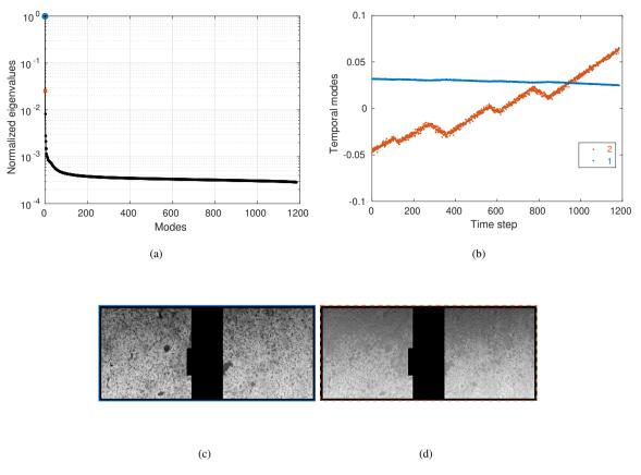
**Figure 13:** (a) Normalized eigenvalues of SVD of  $\tilde{g}$  for the second WST at 600°C (MZ3-S1400G). (b) First two temporal modes and (c-d) corresponding spatial modes of the two ROIs used for NOD measurements (Figure 5)
