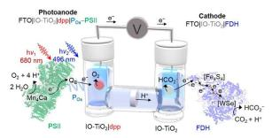
Figure 5 schematic view of the tandem cell used by Sokol and coworkers<sup>[82]</sup> to catalyze the photooxidation of water to  $O_2$  at an anode incorporating photosystem II from *Thermosynechococcus elongatus* (left) coupled to the reduction of  $CO_2$  to formate at a cathode
