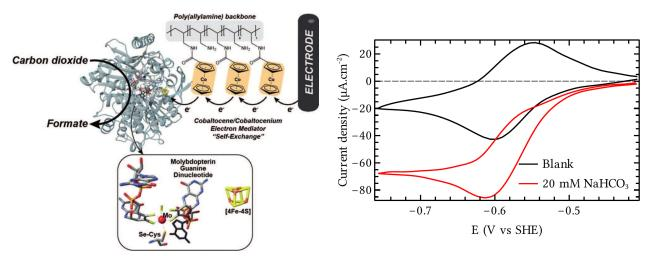
Figure 7: cobaltocene-based redox film incorporating *E. coli* FDH for the reduction of  $CO_2$ . Left: scheme of the device, showing the electron transfer from the electrode to the FDH mediated by hopping across the immobilized cobaltocene moieties. Right: cyclic voltammograms showing the reduction of  $CO_2$ . Data reproduced from <sup>[115]</sup> with permission.
