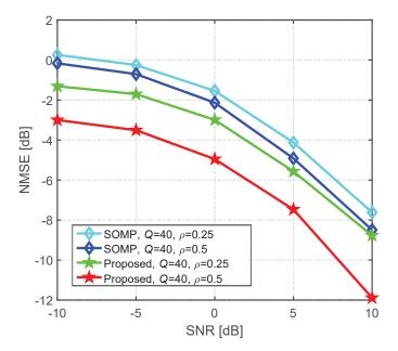
Fig. 15. Channel reconstruction NMSE performance comparison of the proposed MDDL-based channel feedback scheme versus SNRs.
