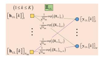
Fig. 4. The proposed fully-connected CCN with the trainable parameters  $\{\Xi_{UL}\}$ , which correspond to the combining matrix  $\mathbf{F}_{III}^{H}$ .
