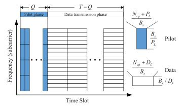
Fig. 1. The proposed frame structure for the communication transmission.
