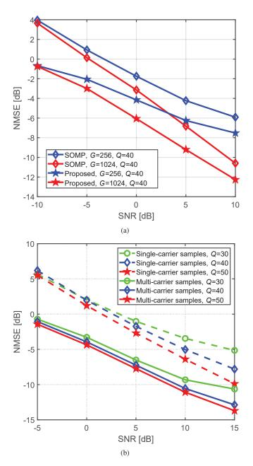
Fig. 13. NMSE performance comparison of the proposed MDDL-based channel estimation scheme versus SNRs, where (a) the effectiveness of the devised redundant dictionary matrix, (b) the effectiveness of the proposed scheme using multi-carrier channel samples to train.
