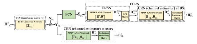
Fig. 6. The block diagram of the proposed MDDL-based downlink channel estimation and feedback solution, where the green and yellow block diagrams represent that the modules are processed at the users and the BS, respectively.
