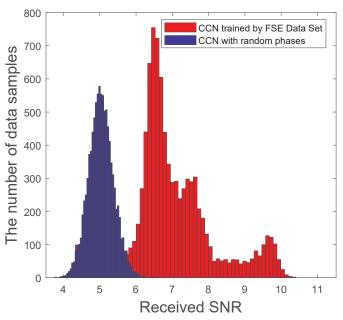
Fig. 18. The received SNR distributions at the user side using different CCNs.
