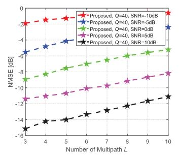
Fig. 9. NMSE performance comparison of the proposed scheme versus the number of multipath  ${\cal L}.$
