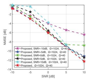
Fig. 10. NMSE performance comparison of the proposed scheme trained at the different SNRs.
