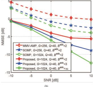
Fig. 14. NMSE performance comparison of the proposed MDDL-based channel estimation scheme versus SNRs, where (a) phase shift quantization, (b) analog-to-digital converter (ADC) quantization.
