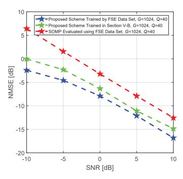
Fig. 17. NMSE performance comparison of different channel estimation schemes versus SNRs.
