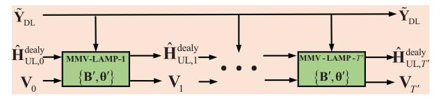
Fig. 7. The proposed FRSN based on MMV-LAMP network with the trainable parameters  $\{\mathbf{B}', \boldsymbol{\theta}'\}$ .
