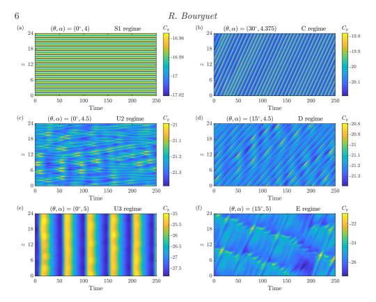
FIGURE 3. Selected time series of the CF force coefficient along the span for (a)  $(\theta, \alpha) = (0^{\circ}, 4)$ , (b)  $(\theta, \alpha) = (30^{\circ}, 4.375)$ , (c)  $(\theta, \alpha) = (0^{\circ}, 4.5)$ , (d)  $(\theta, \alpha) = (15^{\circ}, 4.5)$ , (e)  $(\theta, \alpha) = (0^{\circ}, 5)$  and (f)  $(\theta, \alpha) = (15^{\circ}, 5)$ . Flow regime is specified in each panel.
