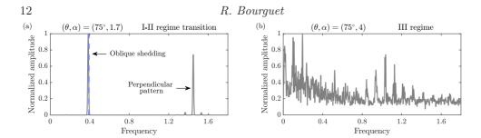
FIGURE 10. Same as figure 5 for  $\theta = 75^{\circ}$ : (a)  $\alpha = 1.7$  and (b)  $\alpha = 4$ . In (a), a blue dashed line denotes the oblique vortex shedding frequency for  $(\theta, \alpha) = (75^{\circ}, 1.5)$  (I regime).
