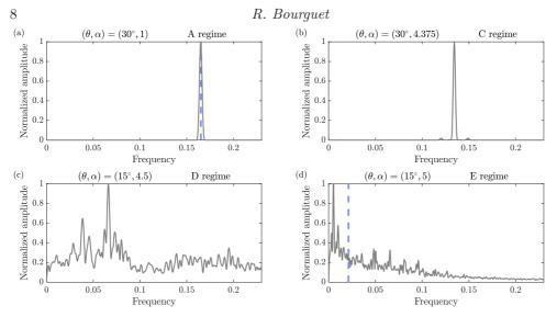
FIGURE 5. Span-averaged frequency spectrum of the CF force coefficient fluctuation for (a)  $(\theta, \alpha) = (30^{\circ}, 1)$ , (b)  $(\theta, \alpha) = (30^{\circ}, 4.375)$ , (c)  $(\theta, \alpha) = (15^{\circ}, 4.5)$  and (d)  $(\theta, \alpha) = (15^{\circ}, 5)$ . The spectral amplitudes are normalized by their maximum value. Flow regime is specified in each panel. In (a,d), a blue dashed line denotes the frequency identified at normal incidence.
