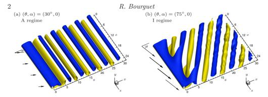
FIGURE 1. Flow patterns downstream of a cylinder inclined in the current at Re = 100, in the absence of rotation: instantaneous iso-surfaces of spanwise vorticity ( $\omega_z = \pm 0.35$ ) for (a)  $\theta = 30^{\circ}$  and (b)  $\theta = 75^{\circ}$ . Arrows denote the oncoming flow. The regime names indicated in the panels will be introduced in §3 and §4. Part of the computational domain is shown.
