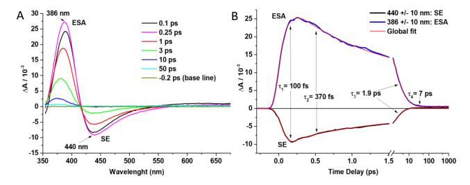
**Figure 5.** Transient absorption spectra. (A) Selected traces for the *E*-2 anion in methanol upon 350 nm excitation. (B) Transient absorption kinetics traces as a function of pump-probe time delay (in ps) observed at probing wavelengths of 386 nm. Both kinetic traces overlap with the result of the global, multiexponential fit (red lines). Four time constants ( $\tau_1$ – $\tau_4$ ) displayed on the graph are required for an accurate fit.
