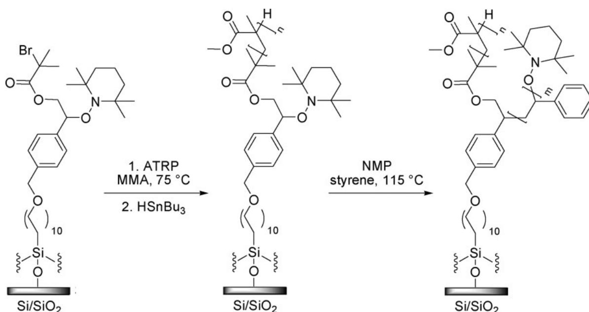
**Figure 13.** Synthetic strategy used to graft mixed Y-shaped PMMA/PS brushes from a self-assembled monolayer of asymmetric bifunctional initiator [110], Copyright 2004. Adapted with permission from the American Chemical Society.
