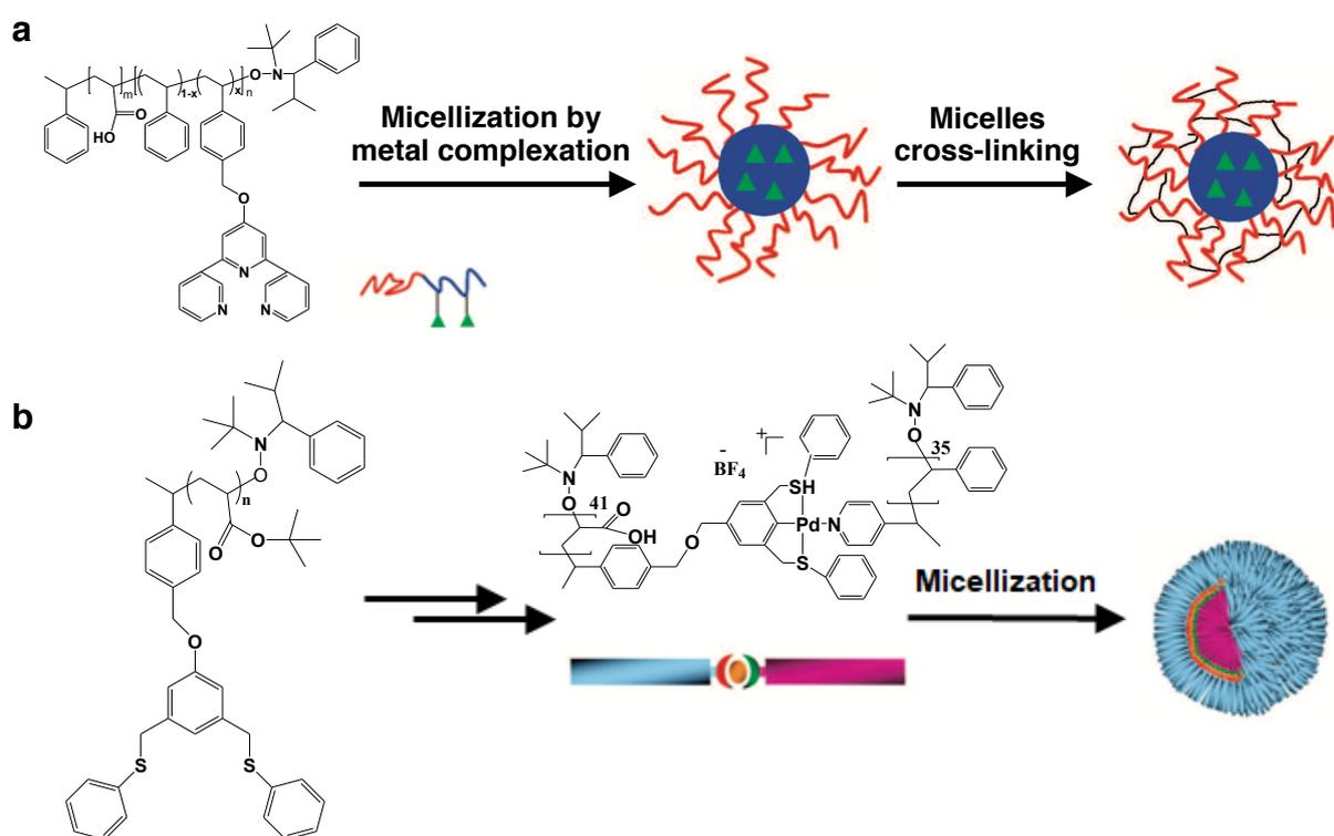
**Figure 25.** Preparation of metallo diblock copolymer-based micelles using functional copolymers synthesized by NMP. Panel a) illustrates the formation of the functionalized spherical micelles using the terpyridine approach [221] while Panel b) corresponds to the use of block copolymers made from the sulfur-carbon-sulfur pincer ligands [222], Copyright 2008. Adapted with permission from the American Chemical Society.
