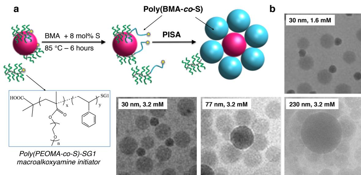
**Figure 33.** a) Scheme illustrating the synthesis of multipod-like silica/polymer composite particles by nitroxide-mediated polymerization-induced self-assembly of block copolymers using a physisorbed brush-like macroalkoxyamine initiator as hydrophilic block, and b) cryo-TEM images of the composite particles obtained in the presence of various silica particle sizes and initiator concentrations [268], Copyright 2015. Adapted with permission from the American Chemical Society.
