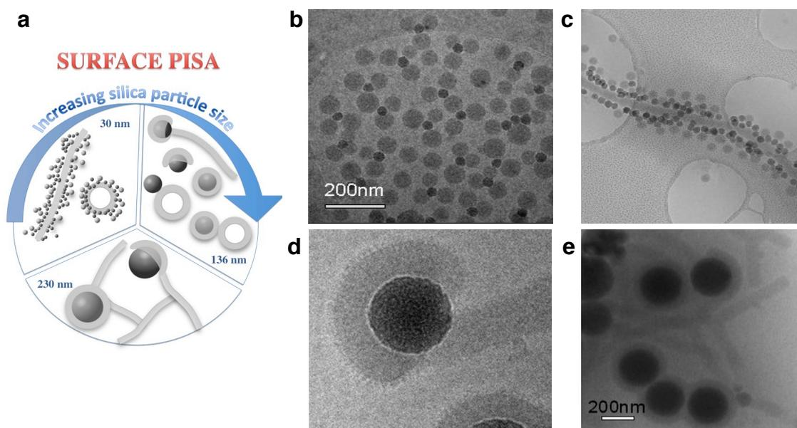
**Figure 34.** Effect of pH and silica particle size on the morphology of silica/polymer composite latex particles synthesized by nitroxide-mediated polymerization-induced self-assembly using a physisorbed brush-like macroalkoxyamine initiator as controlling agent [270], Copyright 2017. Adapted with permission from the American Chemical Society. a) Schematic illustration of the evolution of particle morphology with the silica particle size at  $\text{pH} = 8$ . b-e) Cryo-TEM images of the
