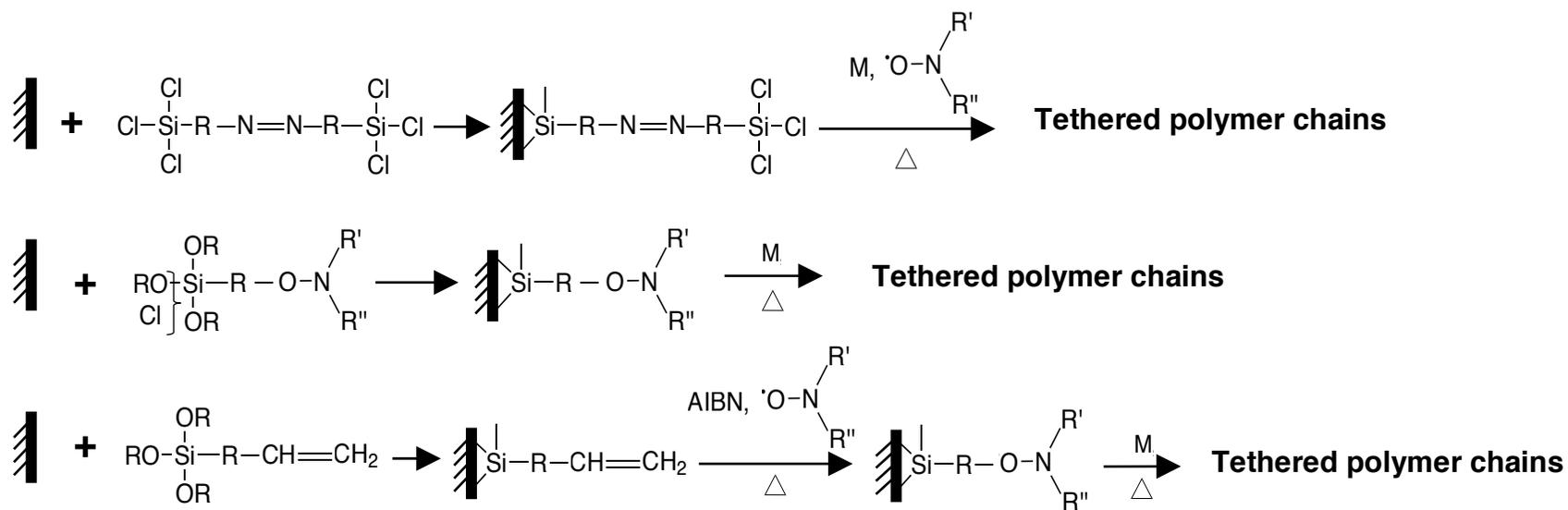
**Figure 6.** Scheme illustrating the growth of polymer chains from inorganic surfaces by SI-NMP using a) a bimolecular or b) a unimolecular initiating system. In scheme c), the alkoxyamine is formed *in situ* by spin trapping radicals produced at the particle surface with a nitroxide.
