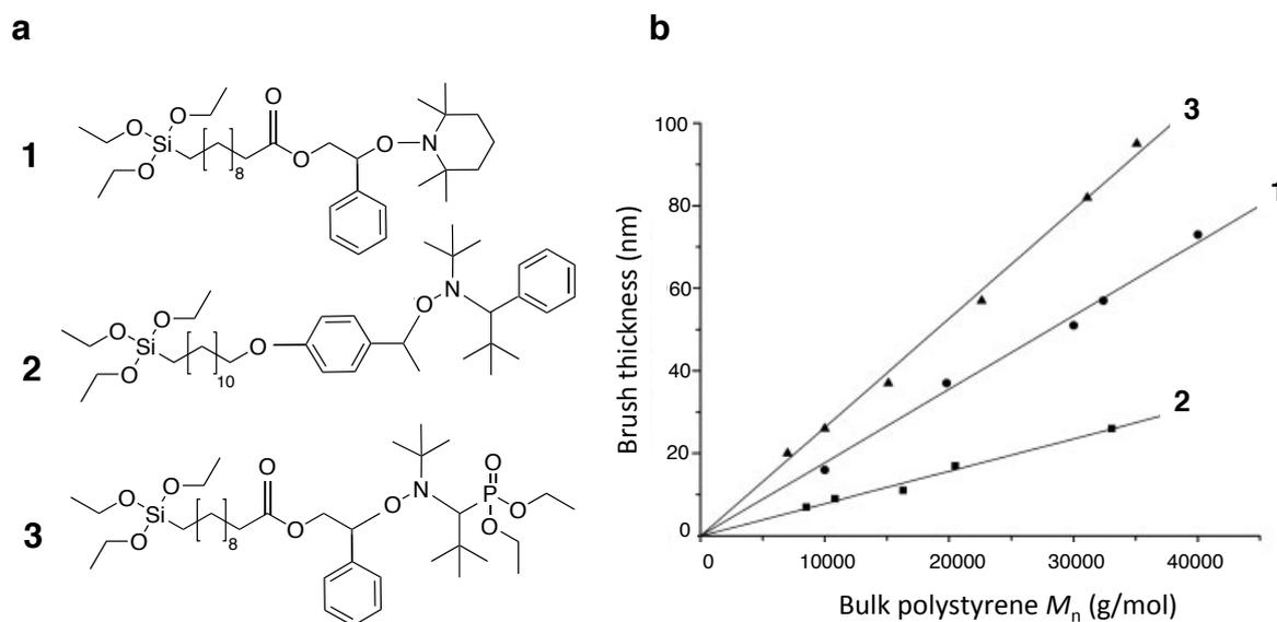
**Figure 9.** a) Chemical formula of the triethoxysilane-terminated alkoxyamines and b) thickness of PS brushes grafted from alkoxyamines 1–3 deposited onto oxidized silicon wafers by the LB technique versus  $M_n$  of the corresponding bulk polystyrenes [116], Copyright 2008. Adapted with permission from Wiley Periodicals, Inc.
