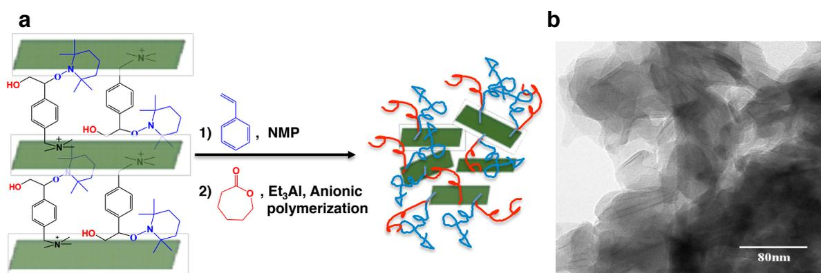
**Figure 28.** a) Schematic illustration and b) TEM image of PS-*b*-PCL/MMT nanocomposites obtained by NMP of styrene followed by anionic ring opening polymerization of  $\epsilon$ -CL using a specifically designed multifunctional silicate-anchored initiator [236], Copyright 2006. Adapted with permission from the American Chemical Society.
