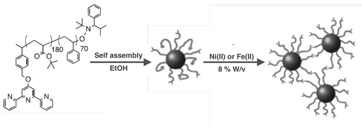
**Figure 26.** Formation of metallo-supramolecular gels through the addition of metal ions to self-assembled block copolymers carrying terpyridine moieties on their outer surface [223], Copyright 2013. Adapted with permission from John Wiley & Sons Inc.
