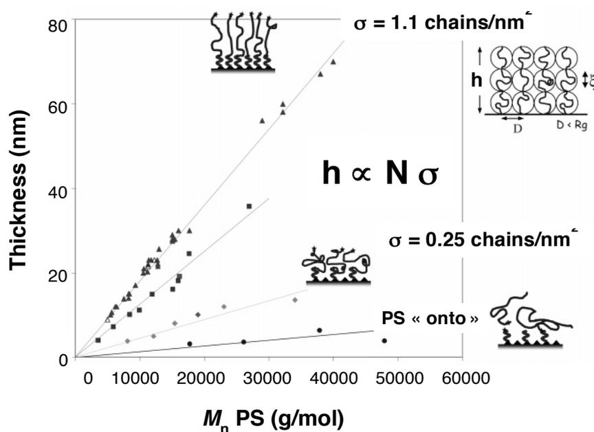
**Figure 8.** Brush thickness measured by ellipsometry in air as a function of the molar mass,  $M_n$  (or chain length  $N$ ), of PS chains grafted from a native silicon oxide surface for different polymer chains grafting densities. An example of grafting onto is also given for comparison [112], Copyright 2005. Reproduced with permission from the American Chemical Society.
