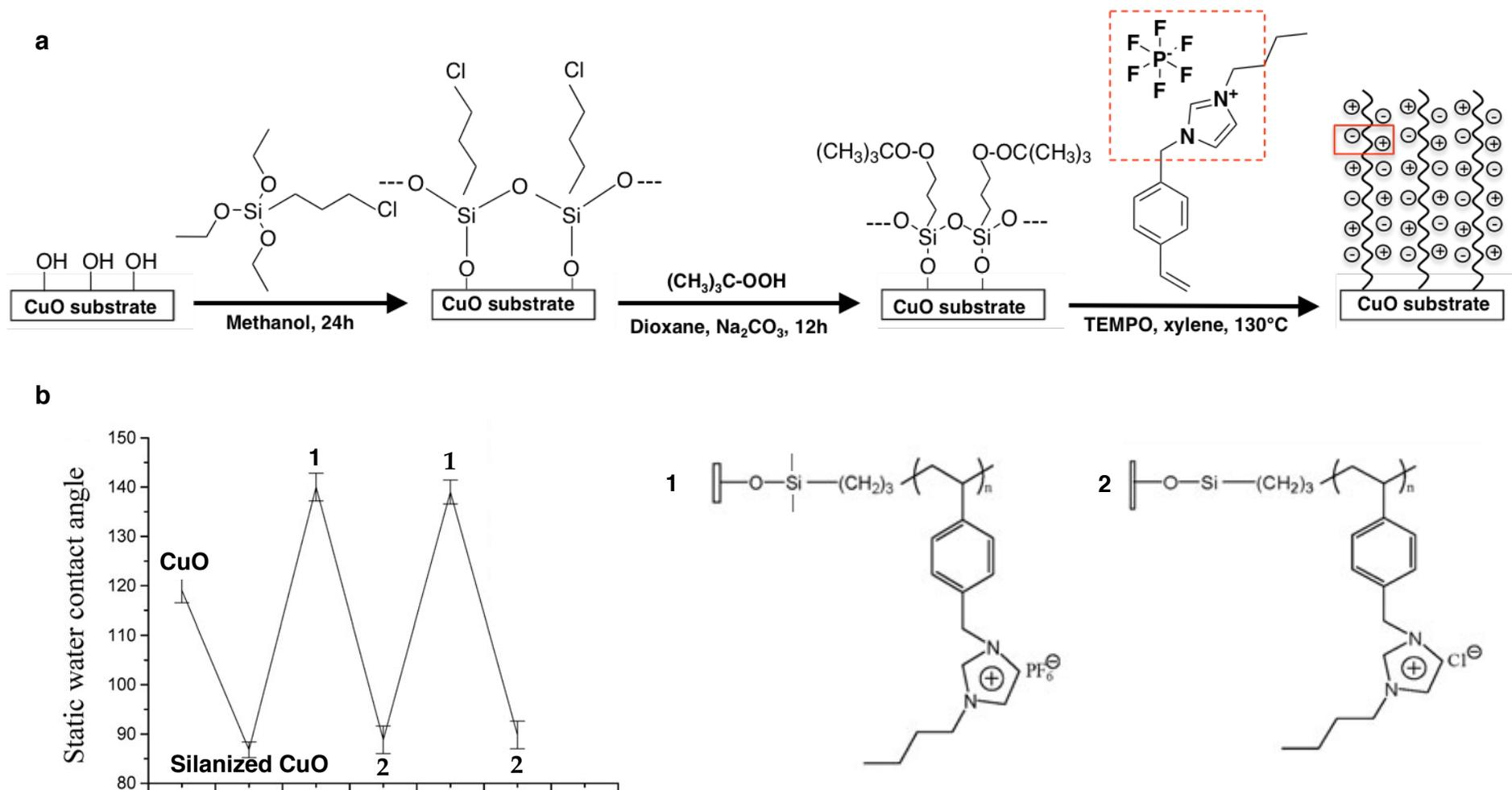
**Figure 12.** a) Synthetic procedure for modifying CuO with a poly(ionic liquid). b) Changes of static water contact angles corresponding to various surfaces of copper sheets [120], Copyright 2012. Adapted with permission from Wiley Periodicals, Inc.
