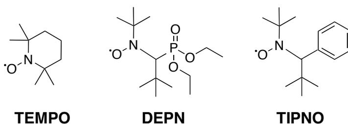
**Figure 5.** Main nitroxyl radicals used in NMP.
