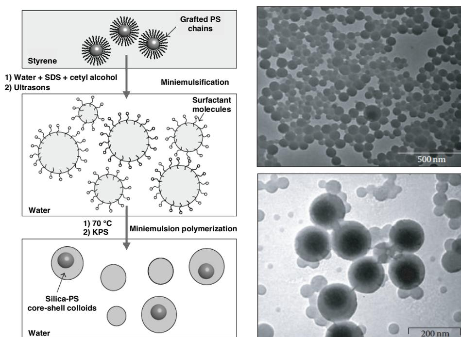
**Figure 32.** a) Scheme illustrating the principle of PS-grafted silica particles encapsulation through miniemulsion polymerization and b) transmission electron micrograph of the produced silica@PS core-shell latex particles [257].
