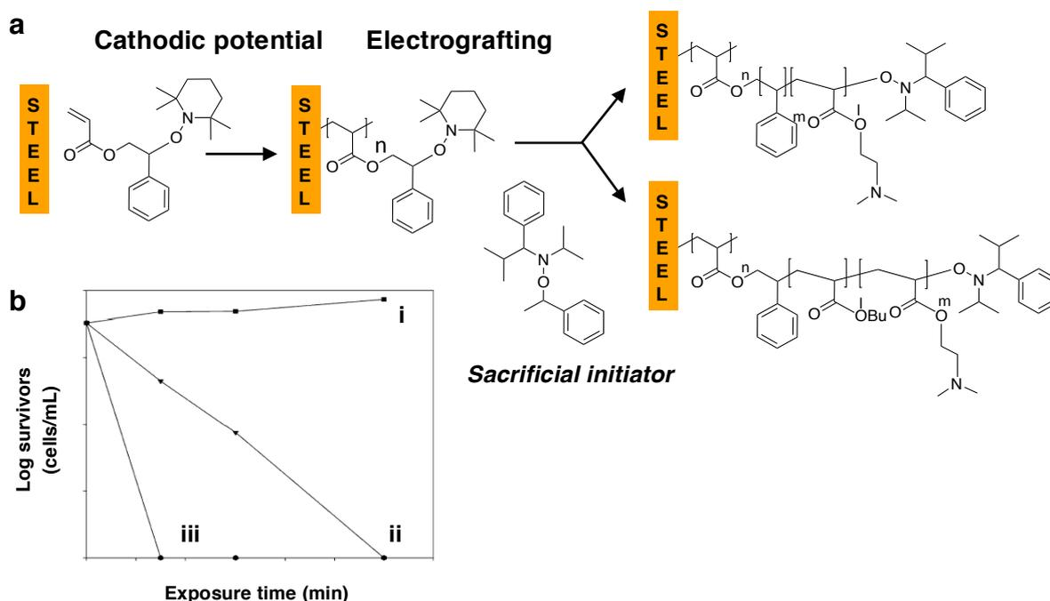
**Figure 22.** a) Synthetic procedure for the grafting of DMAEA-based copolymers onto steel; b) logarithmic plot of the viable cell number of *E. coli* vs the exposure time for i) blank, ii) poly(S<sub>62</sub>-co-DMAEA<sub>38</sub>) quaternized by 1-bromodecane and iii) poly(S<sub>62</sub>-co-DMAEA<sub>38</sub>) quaternized by 1-bromooctane [215], Copyright 2004. Adapted with permission from the American Chemical Society.
