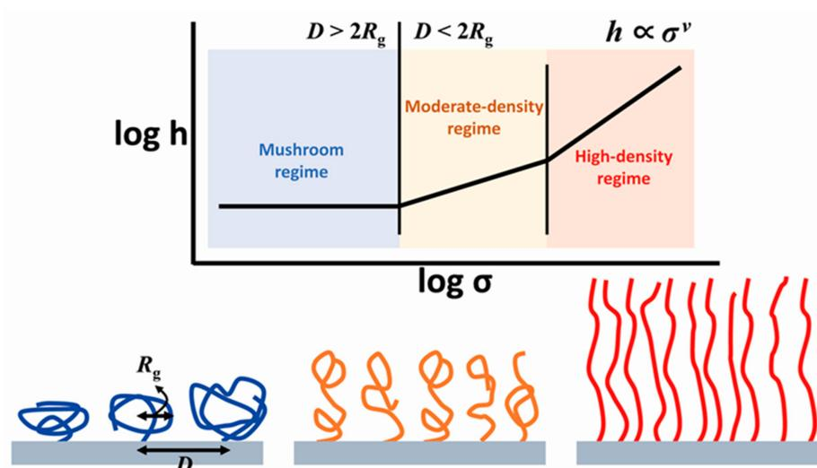
**Figure 2.** Schematic illustration of the three different types of conformations of surface-attached polymers in the case of planar substrates. For  $D > 2R_g$ , the thickness of the film,  $h$ , correlates with the chain density,  $\sigma$ , through the scaling law:  $h \propto \sigma^\nu$ , with the exponent,  $\nu$ , varying with the grafting density and the solvent quality [47].
