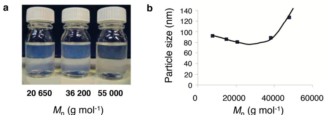
**Figure 29.** a) Digital photographs of PS-grafted Laponite® suspensions in THF at 2 wt% loadings and b) evolution of the hydrodynamic diameter of the hybrid particles as a function of the molar mass of the grafted PS chains determined by SEC [238], Copyright 2007. Reproduced with permission from the American Chemical Society.
