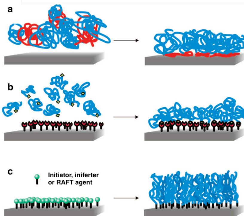
**Figure 1.** Schematic illustration of the three main techniques used to attach polymer chains on inorganic substrates. a) Grafting onto, b) grafting through and c) grafting from. [13], Copyright 2009. Reproduced with permission from the American Chemical Society.
