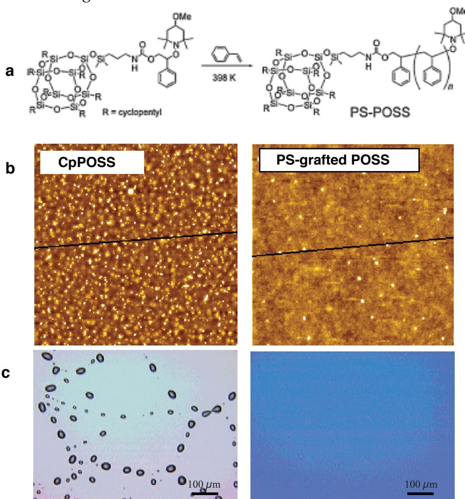
**Figure 27.** a) Scheme for synthesis of PS-grafted POSS by NMP, b) AFM height images and c) optical micrographs of 124 nm thick CpPOSS/PS<sub>1</sub>/PS<sub>2</sub> and PS-grafted POSS/PS<sub>2</sub> blend films annealed at 423K for 3 h (at constant POSS weight content) [230], Copyright 2006. Adapted with permission from the Chemical Society of Japan.
