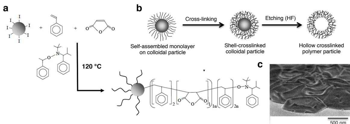
**Figure 18.** a) Preparation of maleic anhydride-functionalized nanoparticles, b) synthetic scheme for the preparation of hollow crosslinked polymer nanocapsules using the silica core as sacrificial template and c) FESEM image of crosslinked poly(styrene-*co*-maleic anhydride)-modified nanocapsules after removal of the silica core by chemical etching with HF [168], Copyright 2002. Adapted with permission from Wiley Periodicals, Inc.
