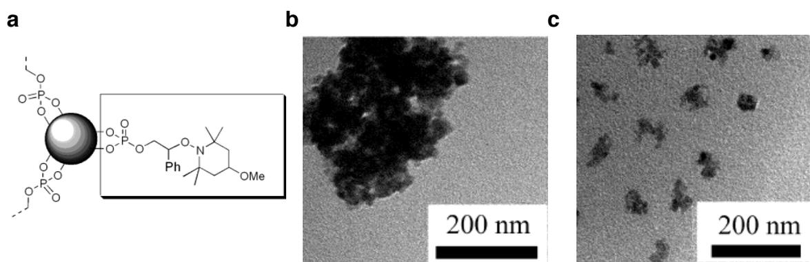
**Figure 21.** a) Grafting of a phosphonic acid-terminated alkoxyamine initiator onto iron oxide particles and b, c) TEM images of b) unmodified and c) PS-modified magnetite particles, dispersed in  $\text{CHCl}_3$  (concentration =  $0.01 \text{ g L}^{-1}$ ) [210], Copyright 2004. Adapted with permission from the American Chemical Society.
