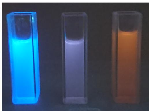
**Figure 8.** Changes in the color of a DMSO solution of **3** ( $c = 1.5 \cdot 10^{-5} \text{ M}$ ) after the addition of 1500 equivalents (middle) and 6700 equivalents (right) of DBU. Photographs were taken in the dark upon irradiation with a hand-held UV lamp ( $\lambda_{\text{exc}} = 366 \text{ nm}$ ).
