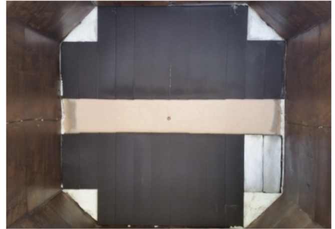
Fig. 11. Assemble of the rigid insulation panel with the flux sensor in the middle.
