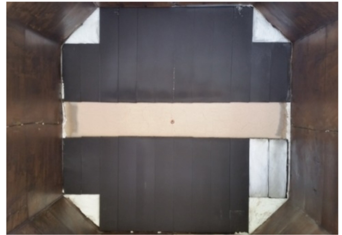
Fig. 11. Assemble of the rigid insulation panel with the flux sensor in the middle.
