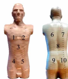
FIG. 6. Positions of the RPL reference dosimeters on the anthropomorphic phantoms.
