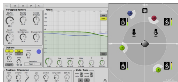
Figure 6: Graphical user interface for spat5.oper (high-level perceptual control for spat~ ). Perceptual factors for controlling room effect (left); filtering (centre); 2D view of the sound scene (right).
