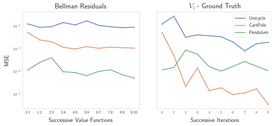
Fig. 1: Convergence of DVP using relative criteria i.e Bellman residuals (left) and absolute criteria i.e difference between value function at each iteration and ground truth (right)
