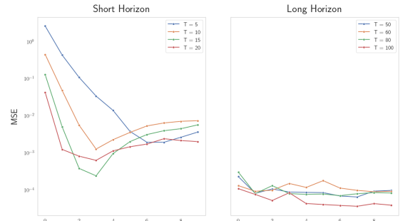
Fig. 3: Evolution of the difference between ground truth value function and different iterations, for short horizons (left) and long horizons (right), shown here for unicycle.
