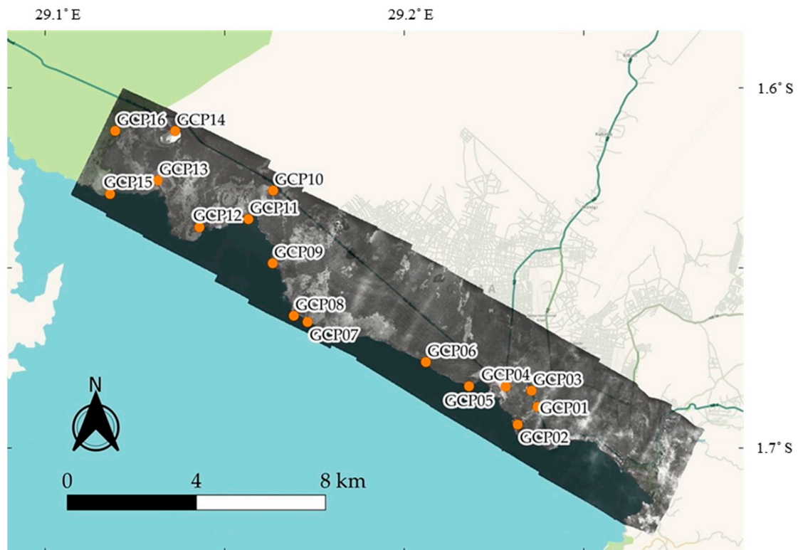
Figure A2. Map showing the distribution of the GCPs used for georeferencing the 1947 orthomosaic of Goma-Gisenyi. The panchromatic image is the orthomosaic. The color map in the background is a Waze map.
