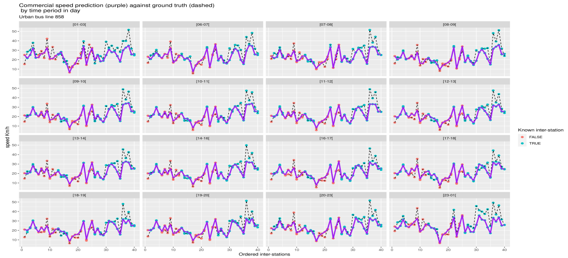
Fig. 3: Speed of urban bus line 858 at inter-stations using micro-learning (purple) vs true speed (dashed). Orange inter-stations where not used by any other bus, i.e. are absent from the training set.
